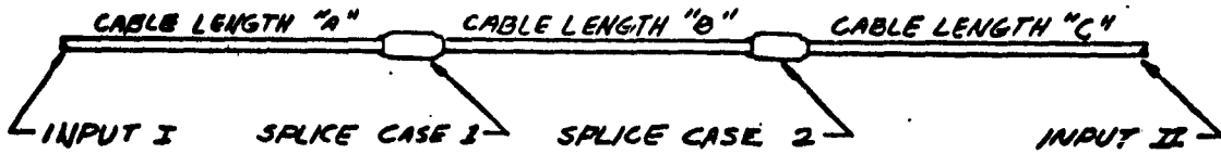
Figure 1. A Run of Pressurized Cable
