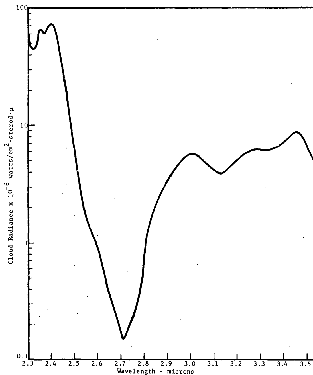
Figure 1: STRATUS DECK 35,000 ft Aircraft altitude 37,000 ft Electrical bandwidth = 0.5 cps Spectral resolution = 0.05 \mu RMS noise 0.075 \frac{\mu \text{ watts}}{\text{cm}^2 \cdot \text{sterod} \cdot \mu}
