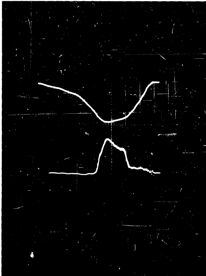
Fig. 21 - Cathode voltage pulse and detected rf pulse at 126 kv. Top trace is cathode voltage. Bottom trace is the detected rf pulse. There are no units of calibration vertically. The horizontal calibration is 2 microseconds per centimeter.
