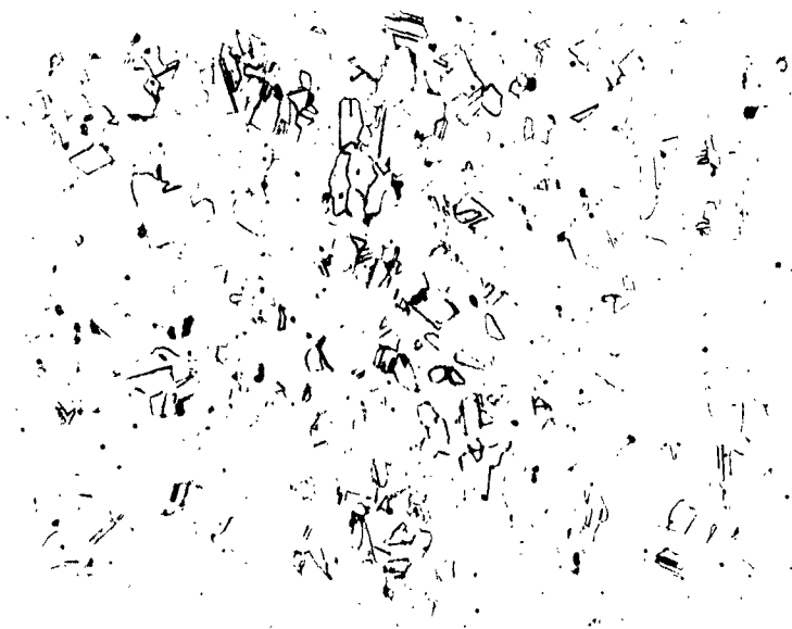
FIGURE 8 UNAFFECTED MIDDLE OF CONTAINER WALL AT 250X
