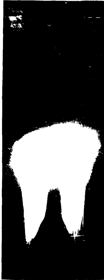
FIGURE 3. TRACE OF A SHOCK WAVE TRANSMITTED THROUGH A POLYURETHANE SAFETY CONTAINER BY THE EXPLOSION OF 5-g NITROGLYCERIN USING AN ELECTRIC S-67 SQUIB AS DETONATOR (Writing speed: 0.6384 mm/ \mu sec)
