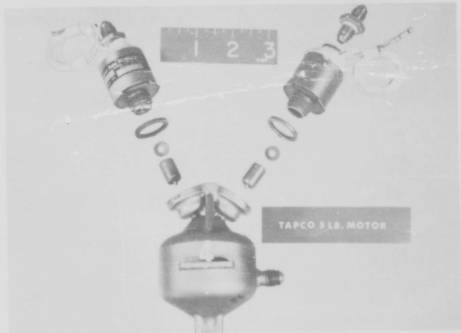
FIG. 2. View of Disassembled TAPCO Pulse Motor.
