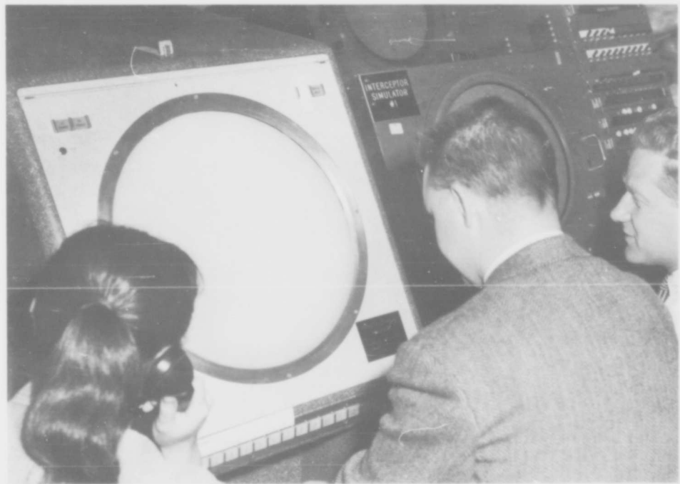
Fig. 2-4. Remote monitor display. The display is located at the Barta Building. The buttons below the display tube's face are for selecting categories.
