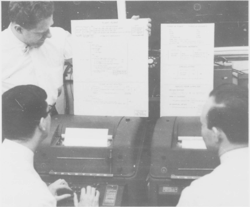
Fig. 2-3. Teletype at the Barta Building. This modified 28 KSR is used for both input and output messages. A similar machine is located at the Boston ARTCC.
