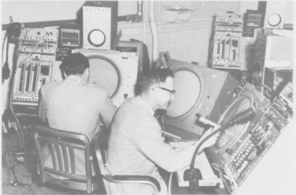
Fig. 3-12. Track monitors and consoles. Two of the four TM positions are shown. Note the wing panels, housing display selection switches (along the top and bottom) and action switches (center). Both TMs are taking light gun actions.
