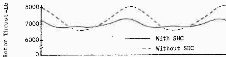
Figure 19. A Comparison of Rotor Thrust With and Without Second Harmonic Control at 40 Knots.
