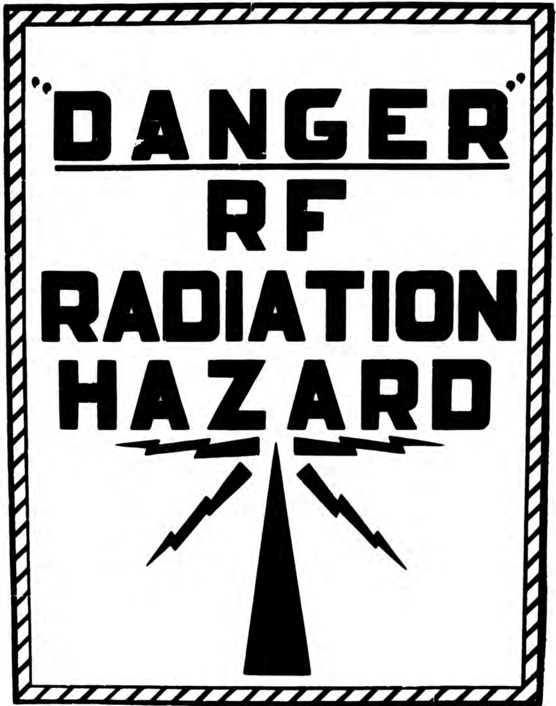
Figure 1-1 Standard Microwave Radiation Hazard Sign
