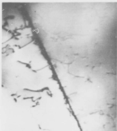
Fig. 91 - Ta(1) strained 4.3% at 293°K Dislocations associated with grain boundary.
