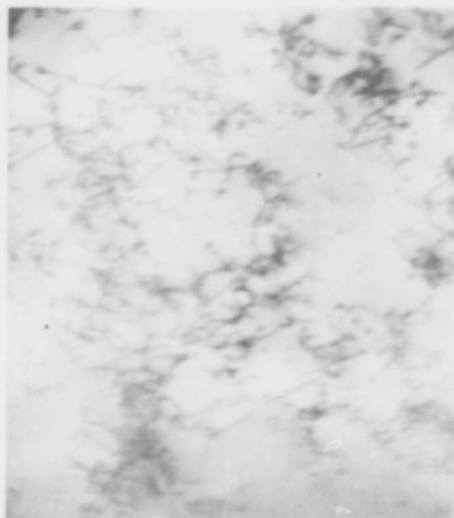
Fig. 93 - Ta(1) strained 9.9% at 293°K Ill defined cell structure.
