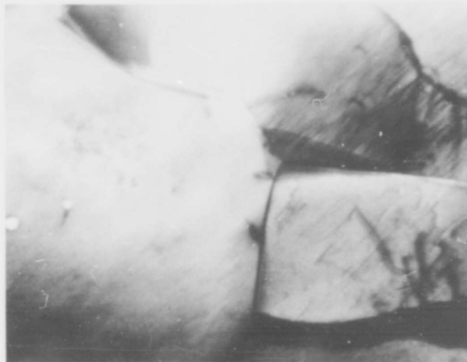
Fig. 48 - Tungsten wire annealed at 1500^{\circ}\text{C} for 30 min. (40,000X).
