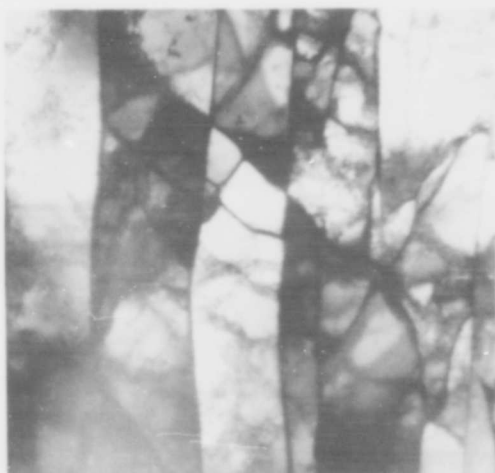
Fig. 5 - Substructure in moderately worked, 46% reduction, molybdenum (Mo-E1) strip, longitudinal section. (a) Light micrograph showing "rectangular" subboundary networks (arrow A) and saw-toothed grain boundary segment (arrow B). (b) and (c) thin-film electron micrographs showing typical microstructure (b), and grain boundary (c).
