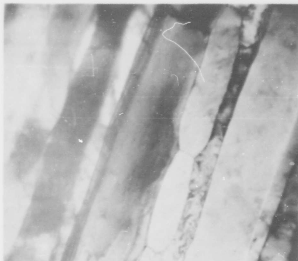
Fig. 49 - Tungsten wire annealed at 900^{\circ}\text{C} for 10 min. (40,000X).
