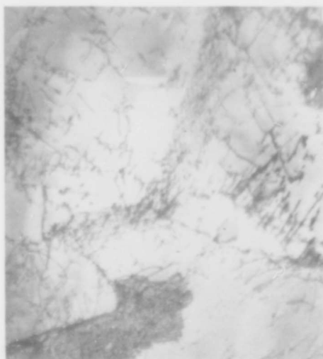
Fig. 97 - Ta(2) strained at 293°K. Exten- sive dislocation networks still remaining after 8.5% strain.
