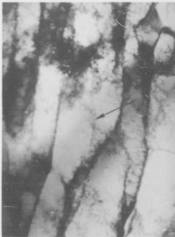
Fig. 6 - Thin-film electron micrograph of moderately worked, 46% reduction, molybdenum (Mo-E1) strip, longitudinal section. Note subboundary formation by dislocation tangles (arrow).
