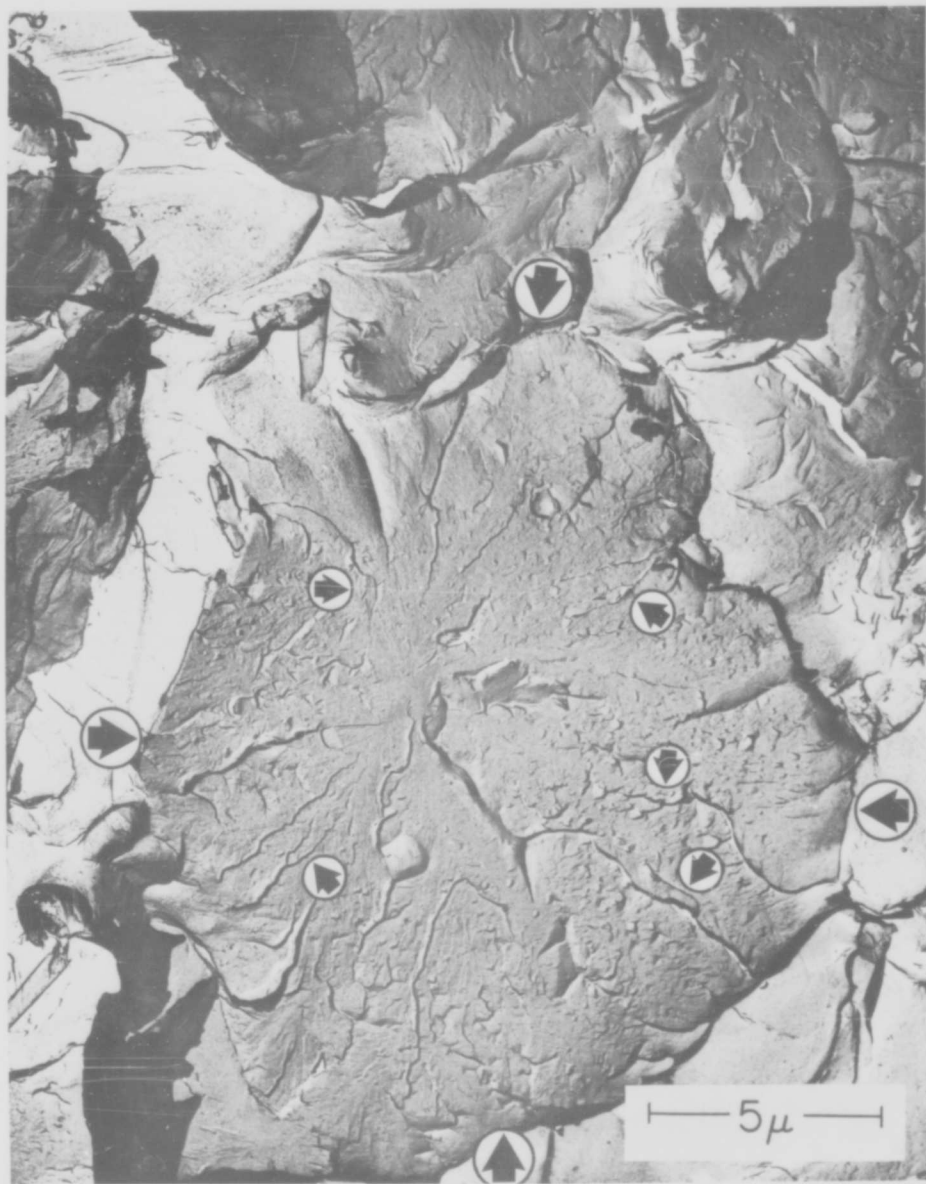
Fig. 5 - Fine scale markings on a quasi-cleavage facet in type 410 stainless steel wire broken at room temperature. The fracture initiation region for this facet is seen just to the left of center of the facet. The large arrows point out the boundaries of the facet while the small arrows indicate river patterns. Cellulose acetate replica technique. 12,000X.
