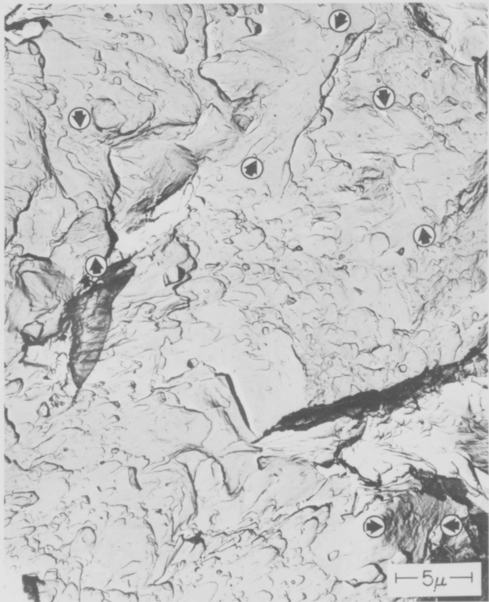
Fig. 10 - Room temperature fracture in 5% Cr die steel showing a few quasi-cleavage facets (between arrows). The main fracture mode is dimpled rupture. Cellulose acetate replication technique. 6,000X.
