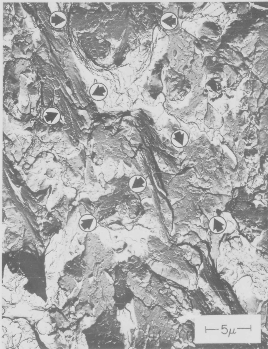
Fig. 6 - Quasi-cleavage in AMS 6434. Specimen broken at liquid nitrogen temperature. Quasi-cleavage facets may be seen between the arrows. Cellulose acetate replication technique. 6,000X.
