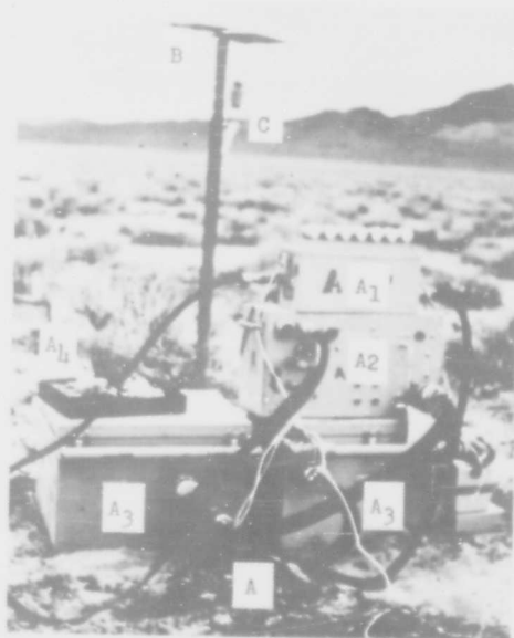
Fig. 2.3—Detail of Lo-Vol air sampler and gummed-tray assembly. (A) Lo-Vol sampler. (A 1 ) filter magazine unit with attached sampling heads. (A 2 ) pump unit. (A 3 ) initial and auxiliary battery boxes. (A 4 ) second series of sampling heads. (B) gummed-tray assembly. (C) film badges.
