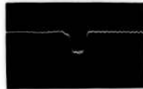
Fig. 44. RF envelope, 0.2- \mu sec pulse duration. Horizontal time scale, 0.2 \mu sec/cm. Horizontal sweep, right to left.
