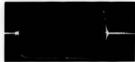
Fig. 55. Gating characteristics of gated IF amplifier. Horizontal scale, 0.5 \mu sec/cm; vertical scale, -0.5 volt/cm (into a 50-ohm load). Carrier frequency, 50 Mcps.
