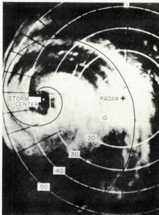
Figure 2.19. An Illustration of the Spiral Overlay Technique in Locating the Center of a Hurricane. (From [34].)
