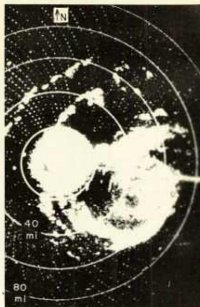
Figure 2.12. A Radar Presentation of Hurricane HELENE Taken During the Deepening State at about -1700 GMT, 25 September 1958 from the APS-20E Radar of a U. S. Navy C-121 (WV-3) Aircraft. The Storm Center at the Time of this Photograph Was about 350 Miles East of Daytona Beach, Florida. (Official Photograph, U. S. Navy.)
