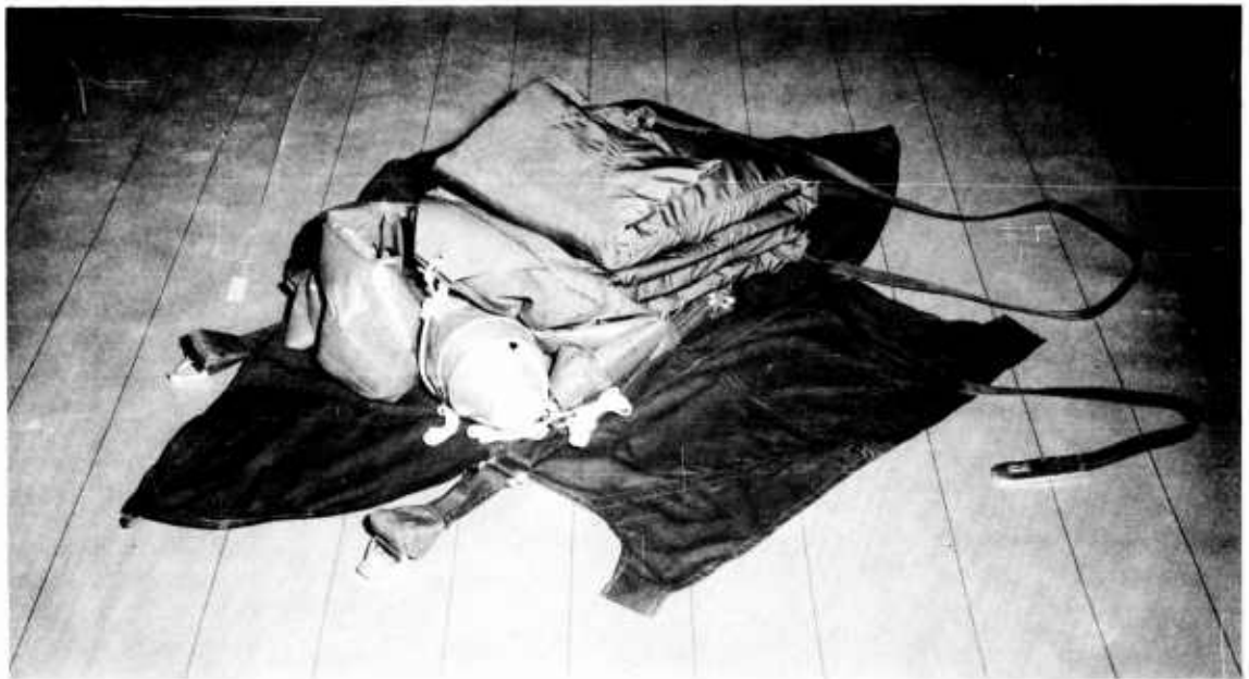
Figure 42 Wing Folded in Back Pack Container
