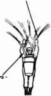
Figure 12 (NO SCALE) SHOWING METHOD OF OBTAINING ROLL CONTROL BY PULLING DOWN ON THE AFT SUSPENSION LINES OF ONE LEADING EDGE ONLY
