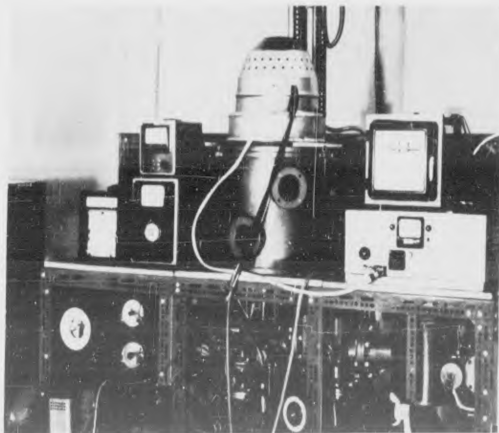
FIGURE 14. Laboratory freeze-dryer with microwave heating system.
