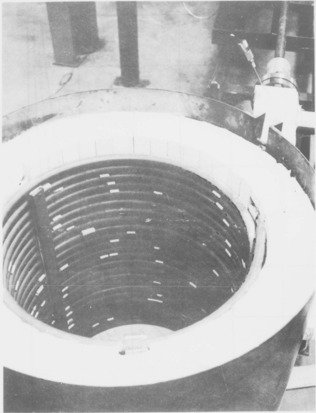
Figure 6. Inconel coil in housing with cover removed
