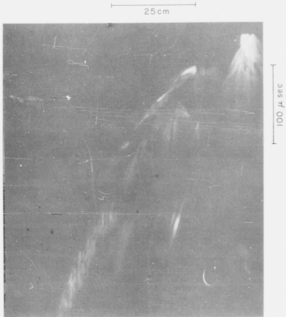
FIGURE 3. - Streak camera record of low-velocity detonation of NG-EGDN in 1/16-inch wall Lucite tube showing unstable propagation.
