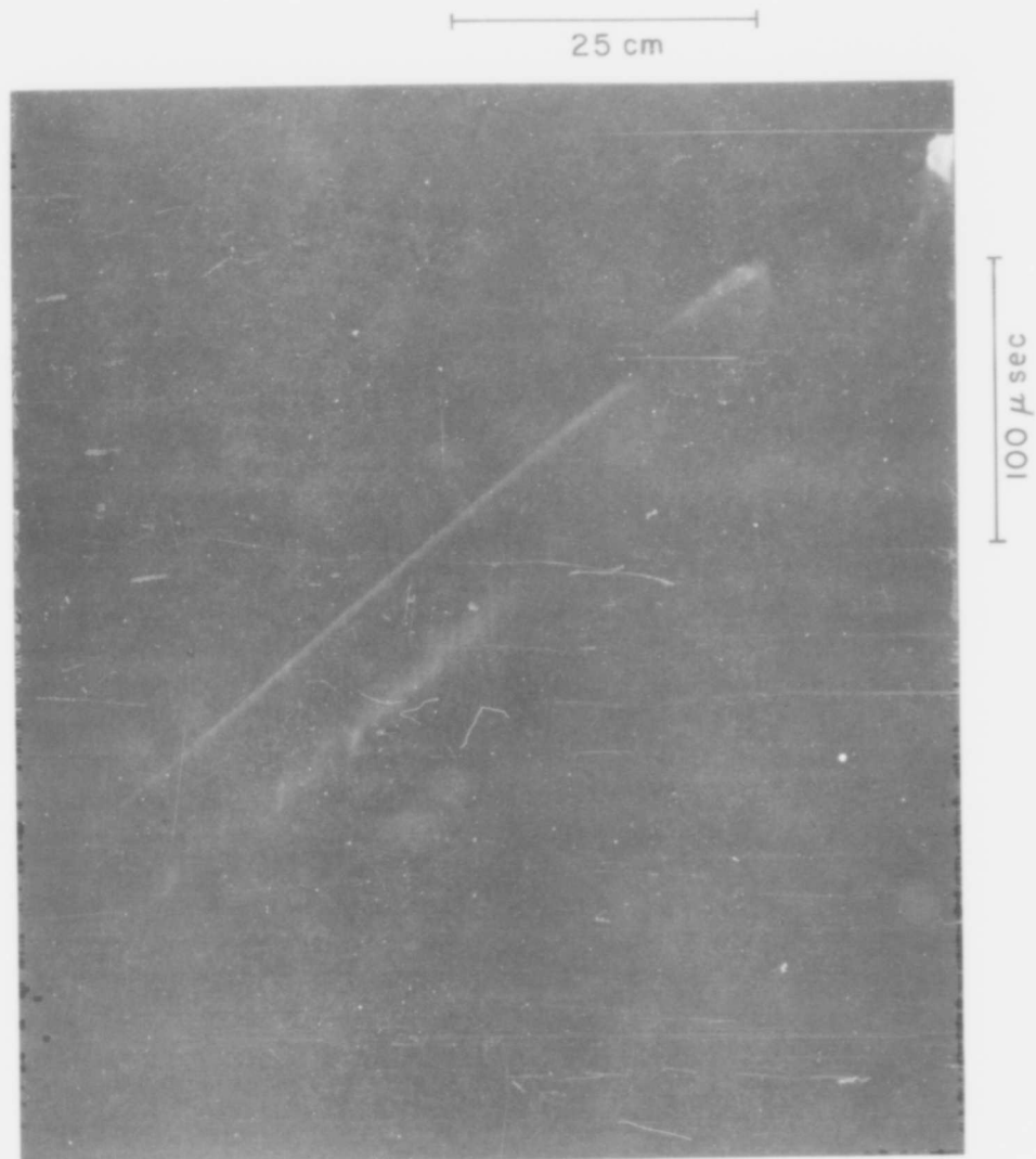
FIGURE 2. - Streak camera record of low-velocity detonation of NG-EGDN in 1/4-inch wall Lucite tube showing stable propagation.
