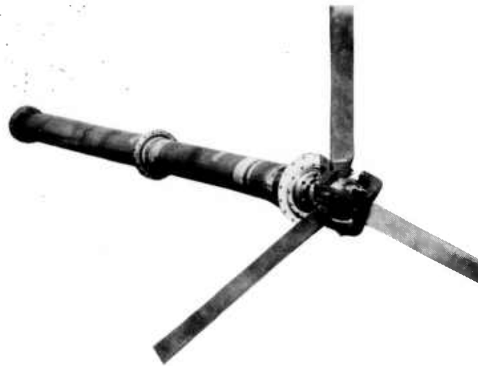
Figure 10. Extension Shaft and Propeller of MARVELETTE.
