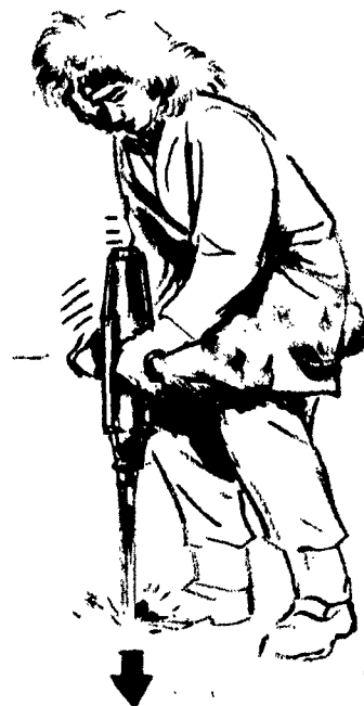
STAKE DRIVING POSITION
