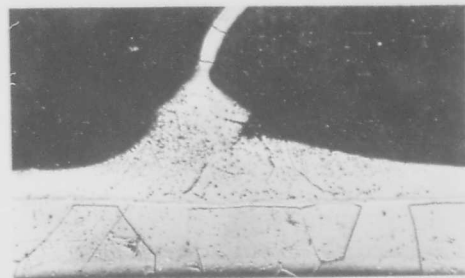
Braze made at 2950° F for 15 min. Specimen was ductile and could be bent without fracture. (200X)
