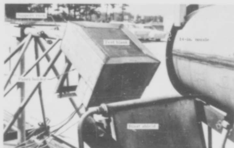
Fig. 148. Hot Gas Facility with Flat Heat Shield Panel Test Fixture
