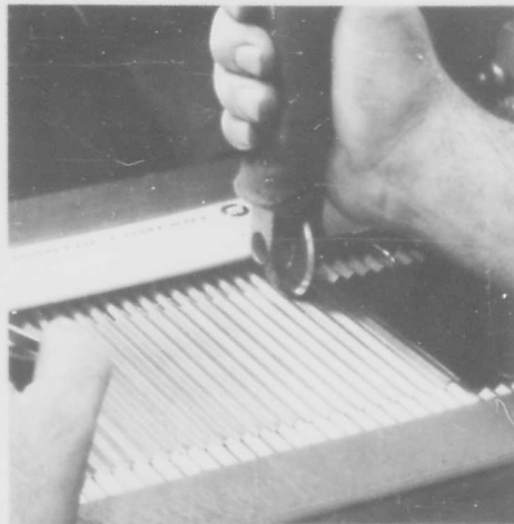
Fig. 25. Tack-Welding Ends of Corrugations in Place
