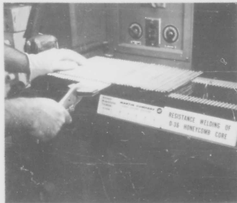
Fig. 24. Tooling for Resistance Welding of D-36 Columbium Honeycomb Core
