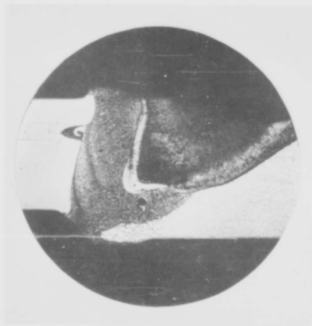
Fig. 91. Photomicrograph of Electron Beam welded D-36 Columbium Joint Attachment Strip to Panel Weld (Magn 75X)
