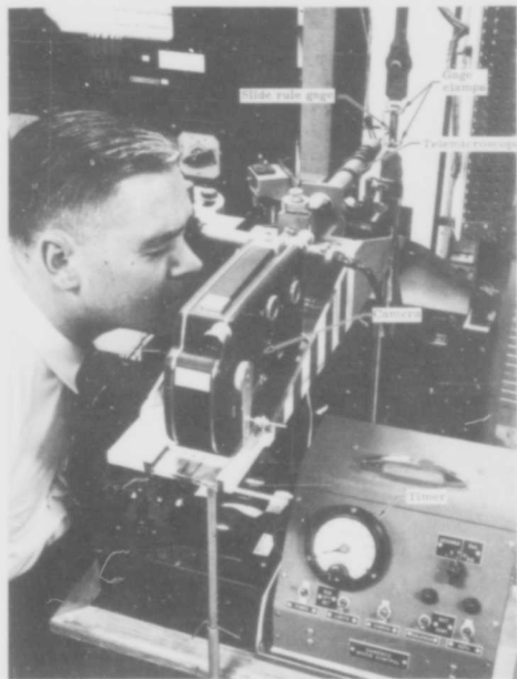
Fig. 168. Tensile Specimen Deflection Measuring System
