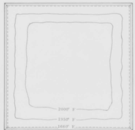
Fig. 124. Temperature Isotherms for 2000° F Compression Panel Temperature Distribution Test
