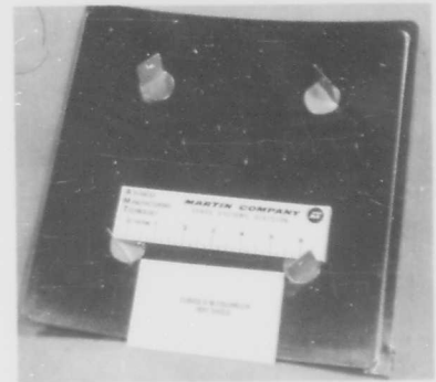
Fig. 90. Curved D-36 Columbian Heat Shield Panel Showing Support Clips
