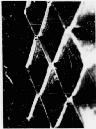
FILLET AND NODE AREAS MAGNIFICATION 3X
