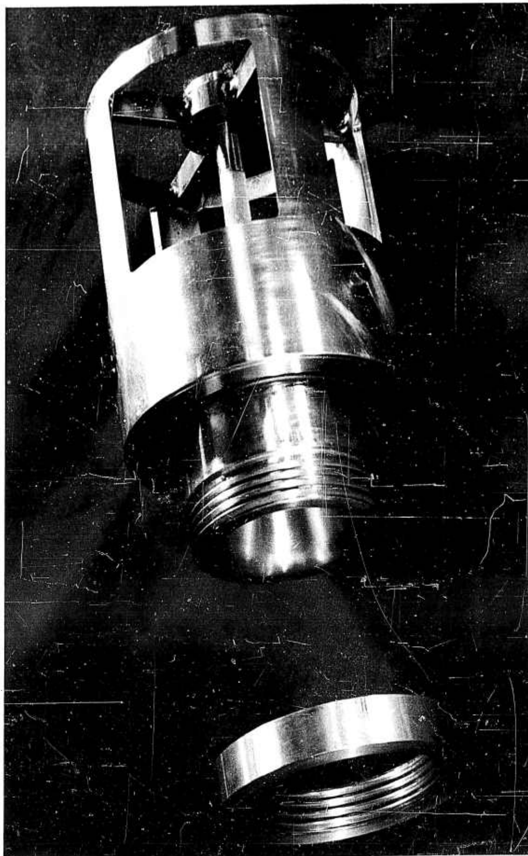
SUPERSONIC NOZZLE WITH PROPELLANT SAMPLE
