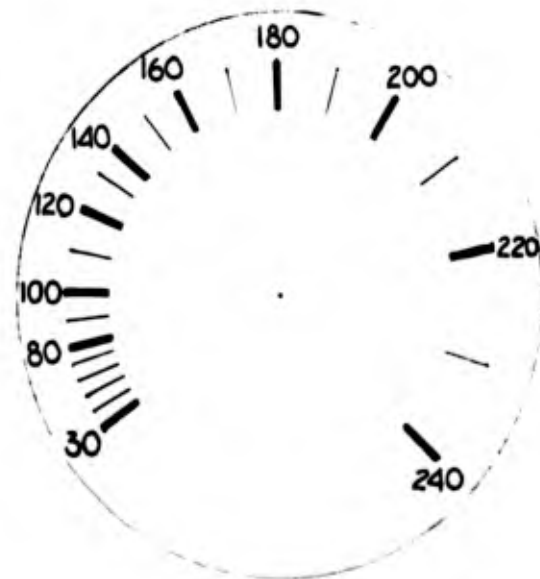
Fig. 3A. PROPOSED LUBE OIL SUMP TEMPERATURE METER
