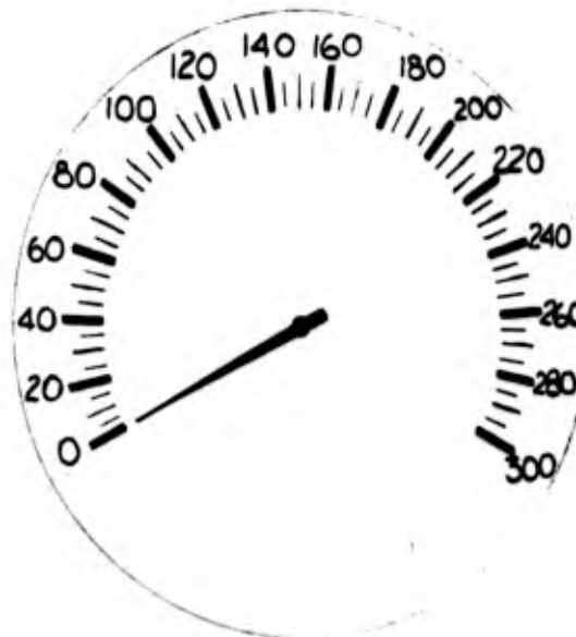
Fig. 5A. PROPOSED LUBE OIL SUMP PRESSURE METER
