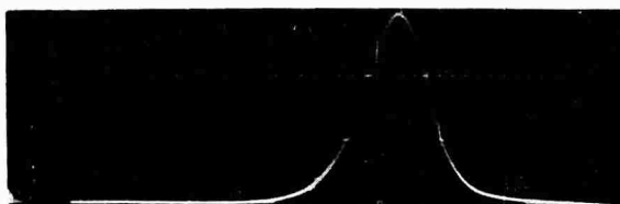
FIGURE 2: SPRF Gamma Dose Rate versus time (Peak value \dot{\gamma}=2 \times 10^7 r/sec) Horizontal Sweep Speed 50 \mu s/cm.
