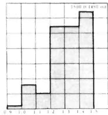
Figure 15. Distribution curves and histograms for the 0.3- to 1.5-sec noise at the surface and at 1500 ft (450 m) in the deep well, Orlando, Florida
