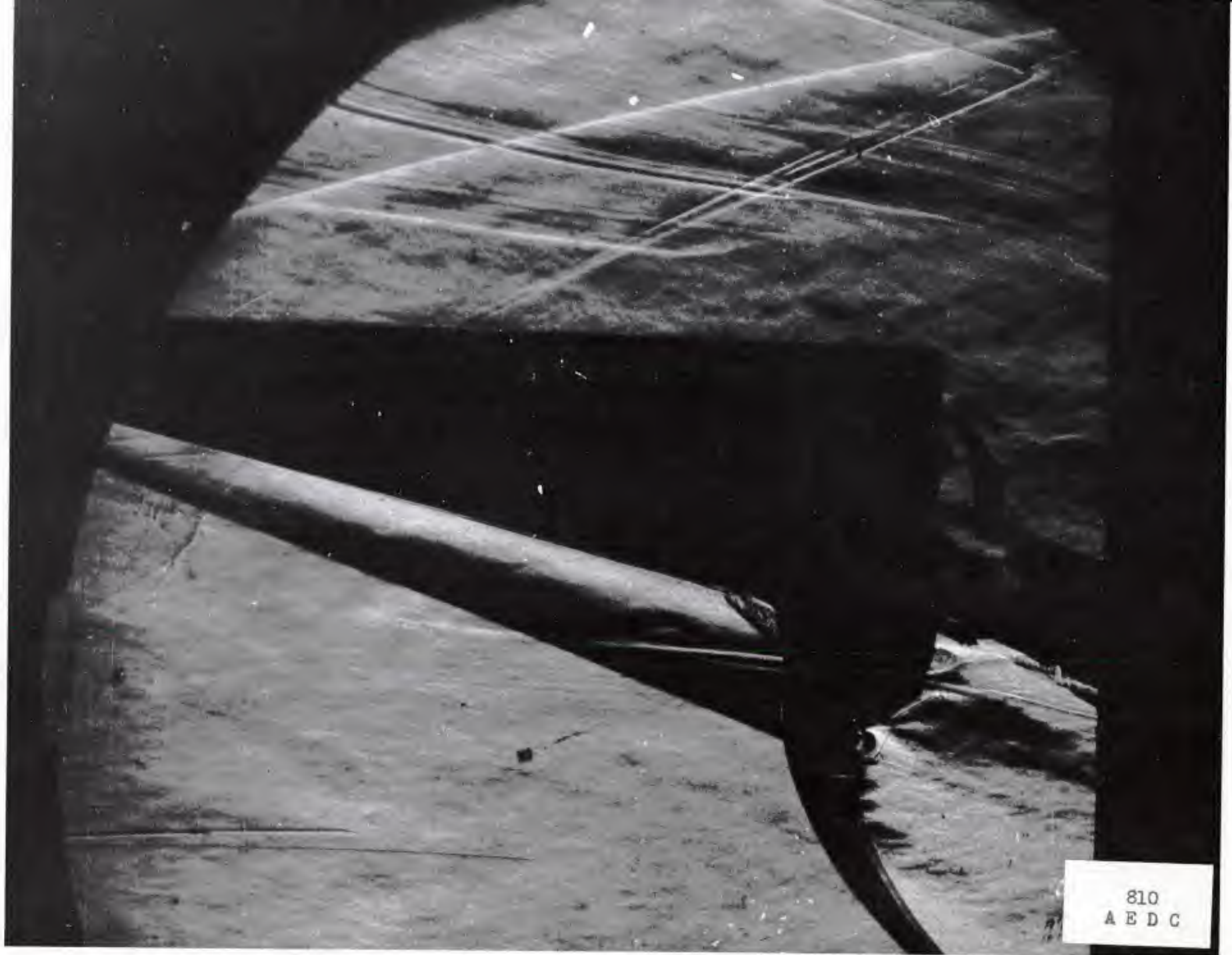
Fig. 23 Schlieren Flow Photograph; \alpha = +14.3^\circ , Bottom Flaps Deflected 40^\circ
