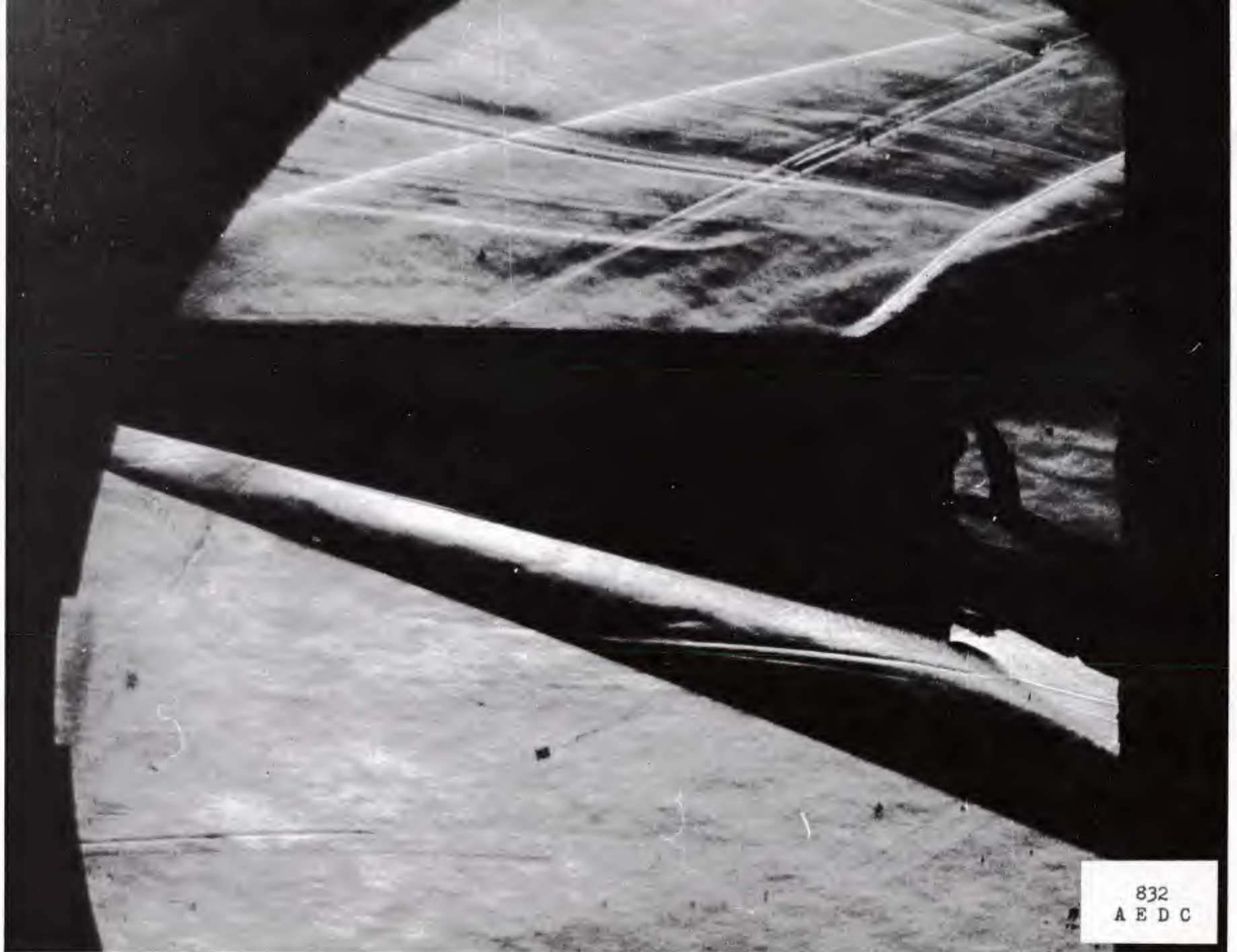
Fig. 19 Schlieren Flow Photograph; \alpha = +14.3^\circ , Upper Left Flap Deflected 40^\circ
