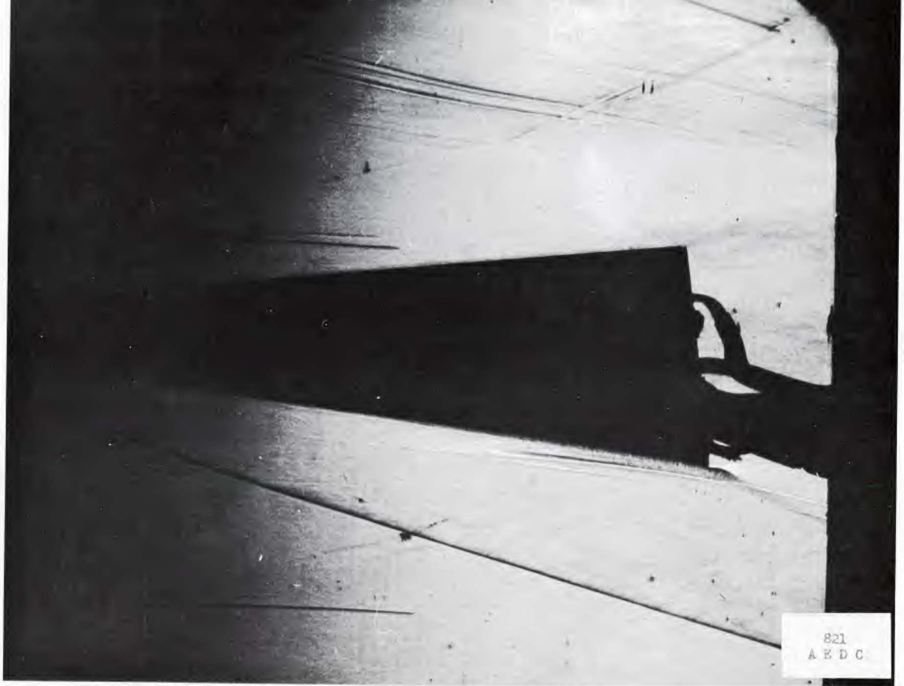
Fig. 17 Schlieren Flow Photograph; \alpha = +7^\circ , No Flap Deflections
