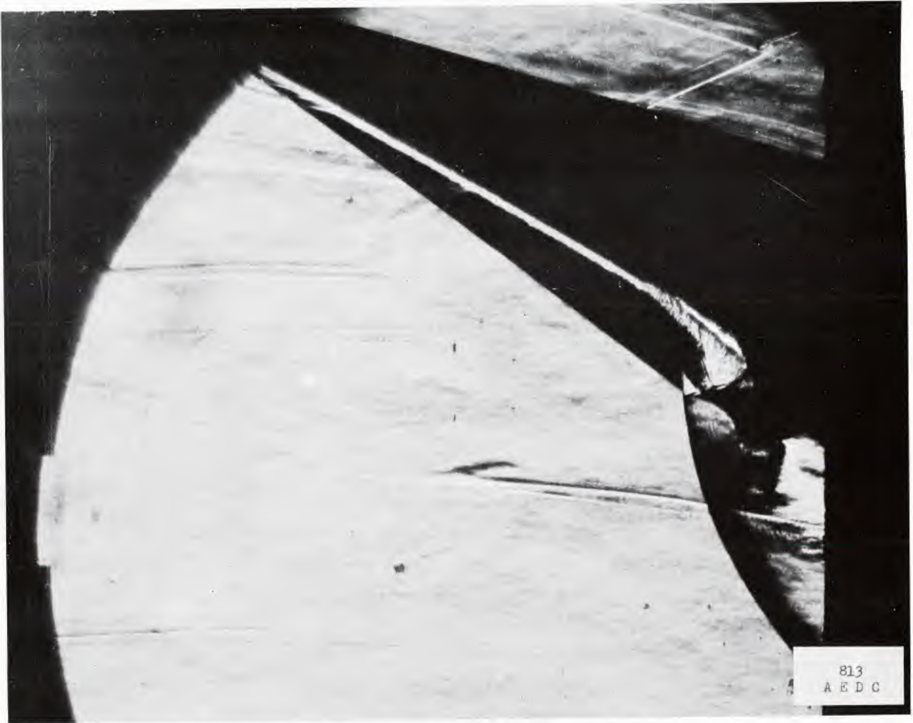
Fig. 26 Schlieren Flow Photograph: \alpha = +30^\circ Bottom Flaps Deflected 40^\circ
