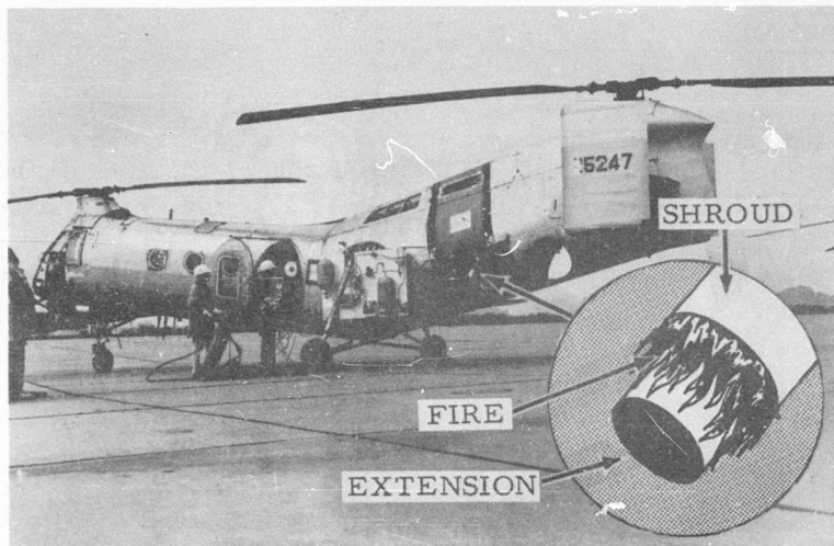
Figure 15. Fire Suppression Test.
