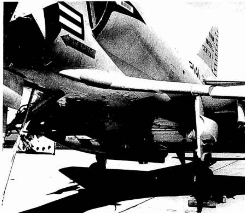
Figure 4. AQM-37A Target and LAU-24/A Launcher on A-4B Aircraft Centerline Station.
