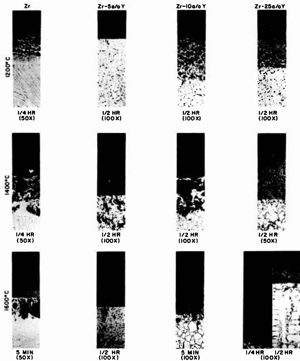
Fig. 26. Microstructures of layers formed in the oxidation of Zr-Y alloys (magnification reduced by 35% in reproduction).
