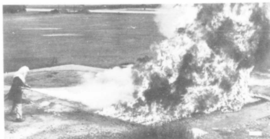
b. Start of attack, using combined-agent unit (initial dry chemical discharge)
