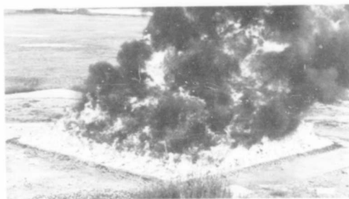
a. Ignition stage of 400 ft 2 large-scale test fire using gasoline fuel
