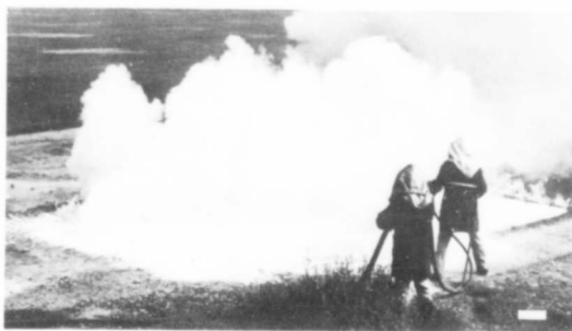
d. Last stages of fire extinguishment (note white vapor-securing cover on fuel)
