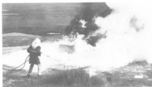
c. Combined-agent discharge on test fire; operator proceeds to right
