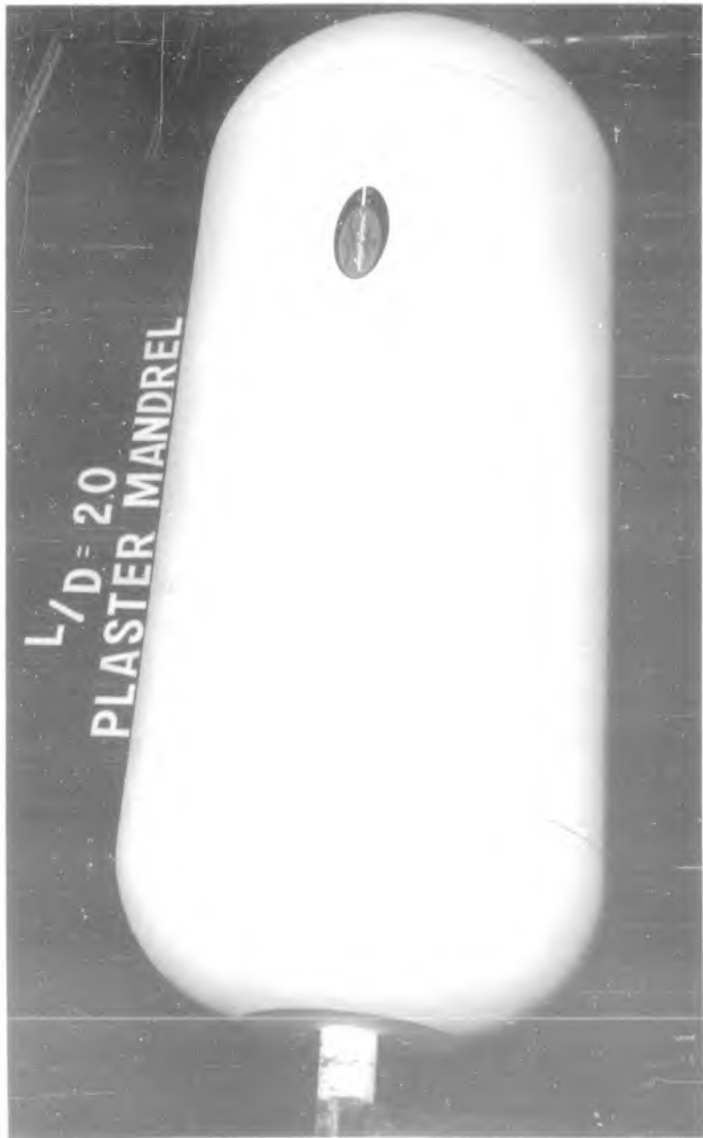
Figure 22. Plaster Mandrel for Model Chamber, L/D_c = 2
