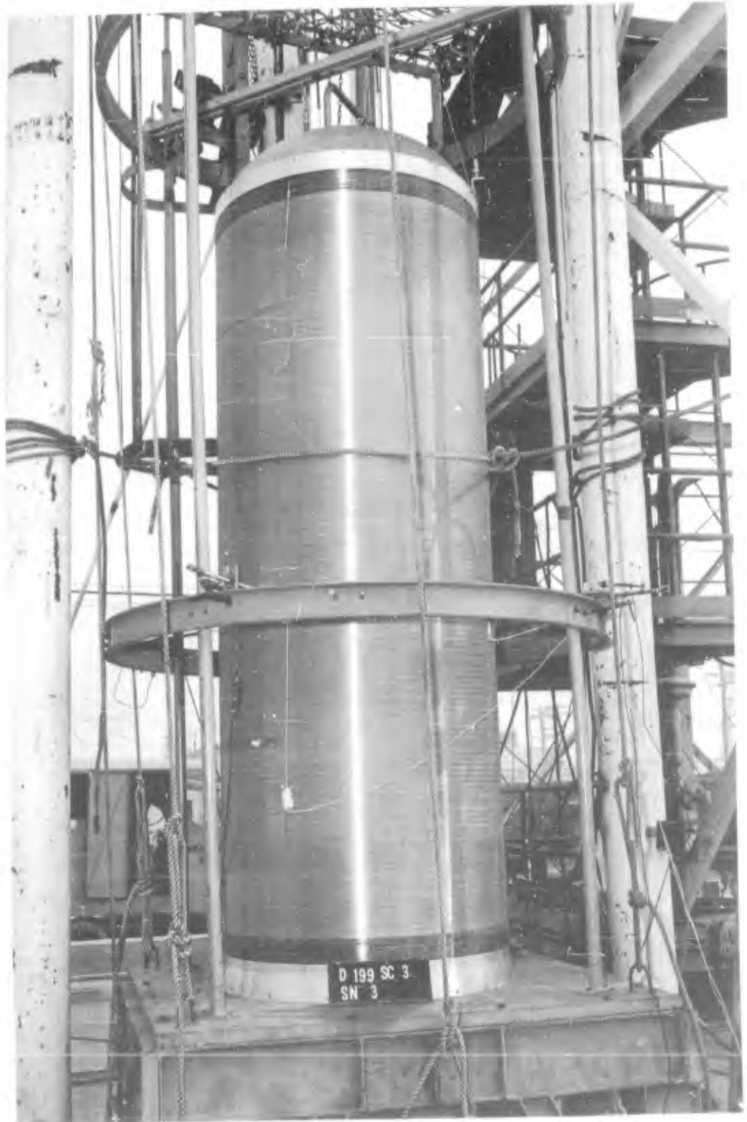
Figure 78. Serial No. 3, 44.3-Inch Chamber, Overall View Prior to Hydrotest
