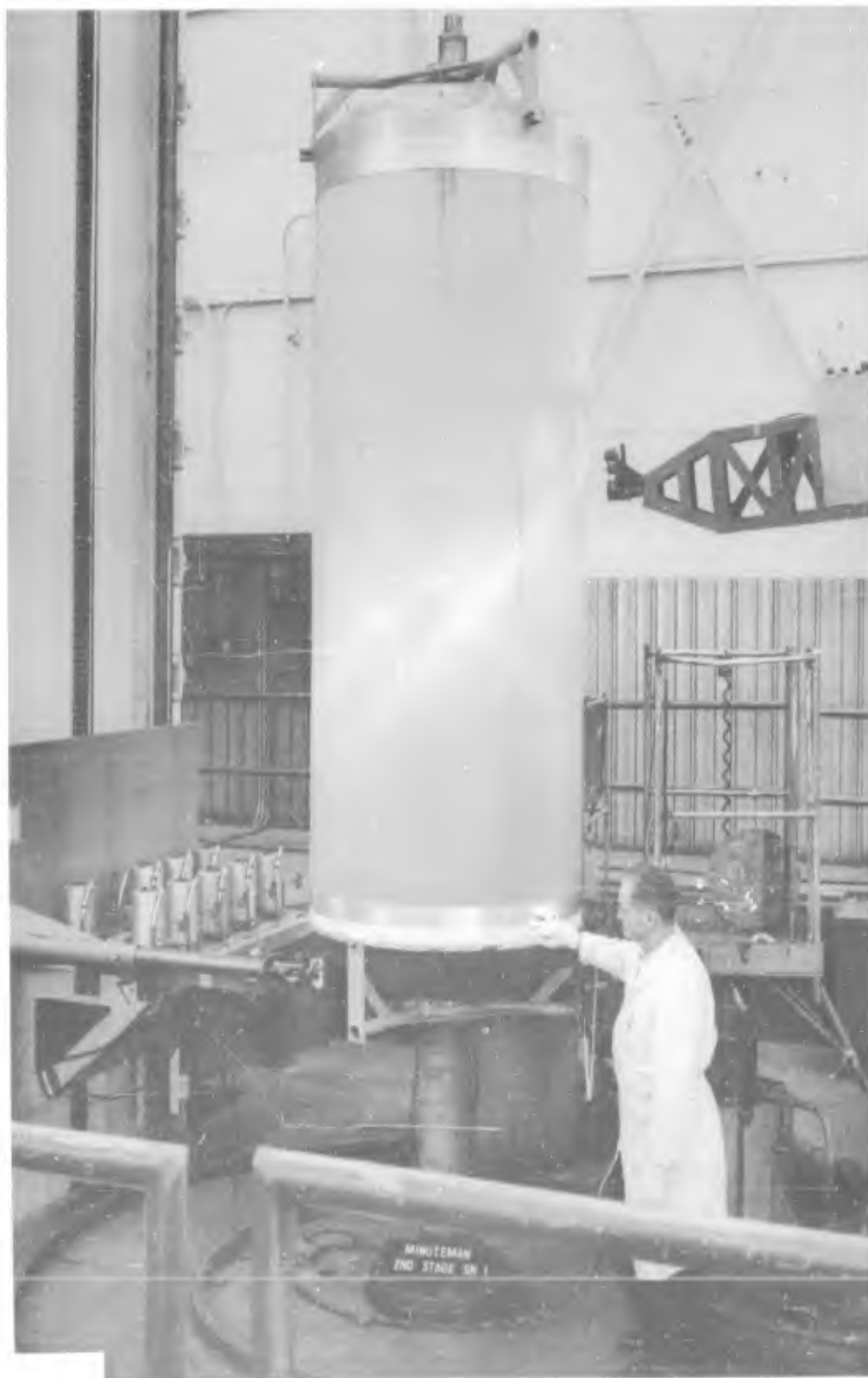
Figure 56. Positioning of Skirts Prior to Hoop-Filament Winding
