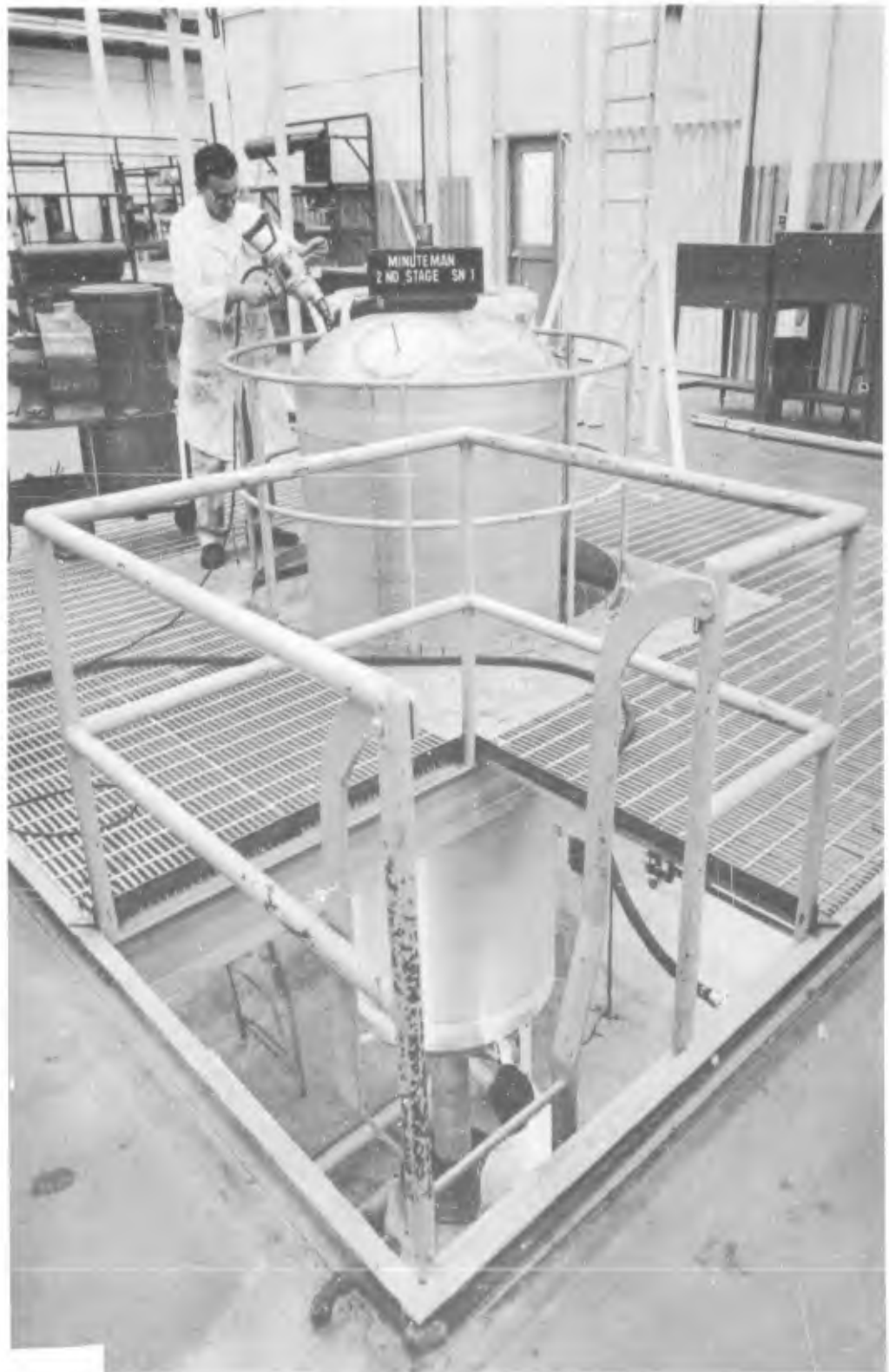
Figure 57. Cutting of Filaments in Aft Nozzle Ports
