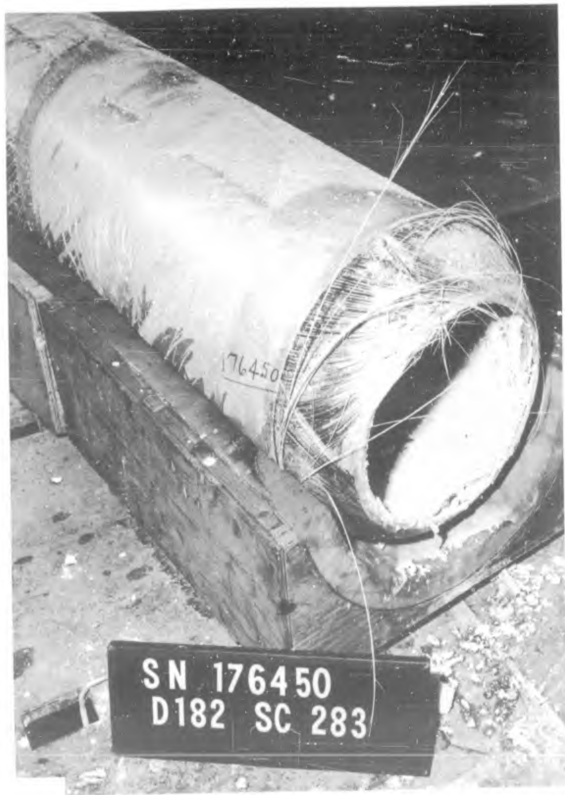
Figure 38. Chamber 176450, After Hydroburst
