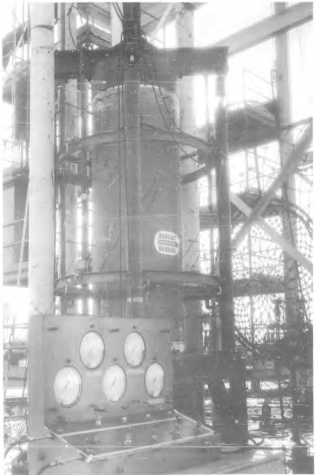
Figure 82. Serial No. 4, 44.3-Inch Chamber, Structural Load Test Setup
