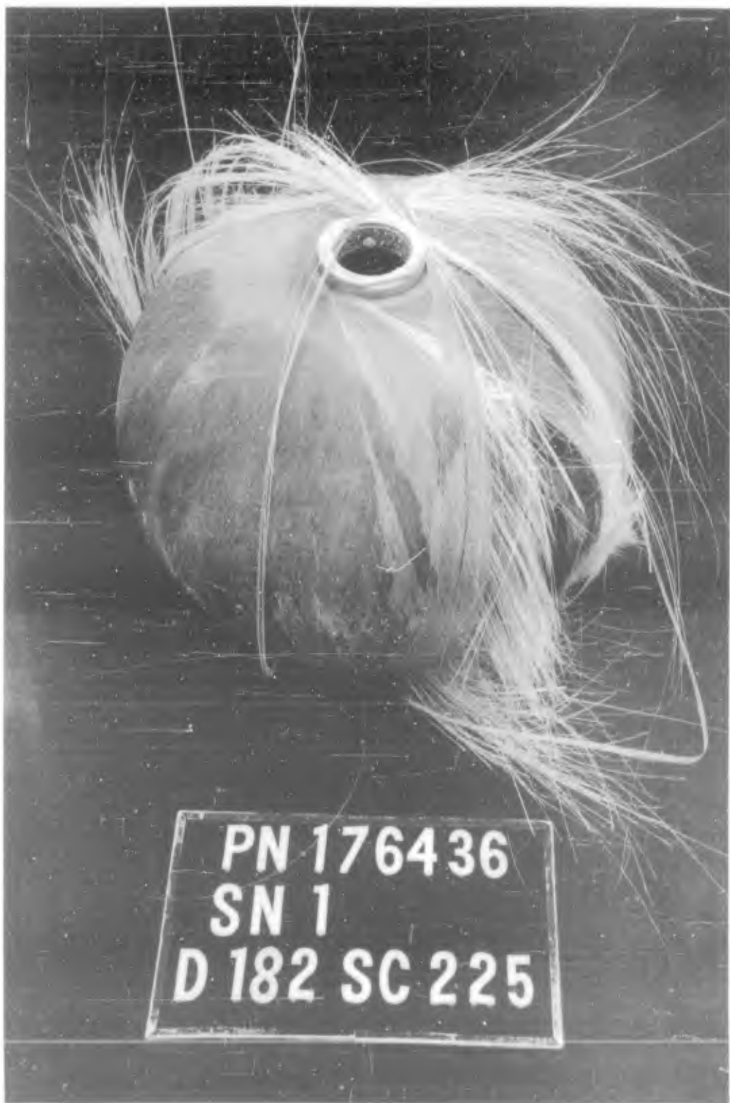
Figure 19. Chamber 176436, After Hydrotest
