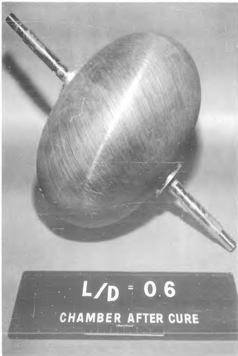
Figure 17. Back-to-Back Model, After Cure
