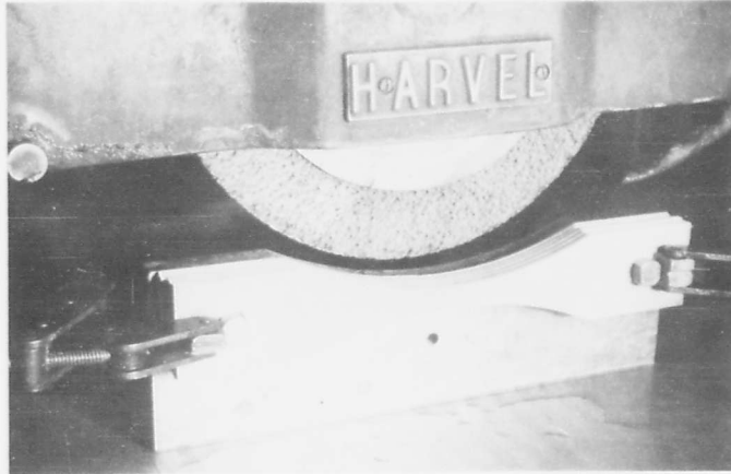
Figure 8. Fatigue Specimens Being Ground to Shape on Precision Surface Grinder
