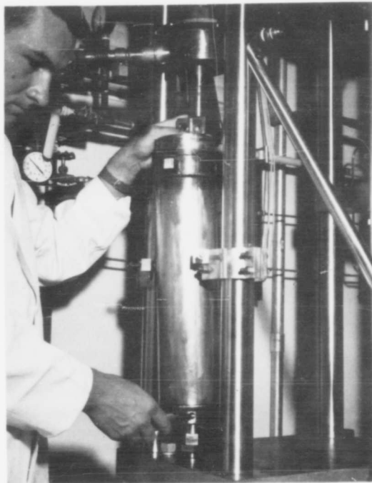
Figure 21. Cryostat Being Installed in Fatigue Machine
