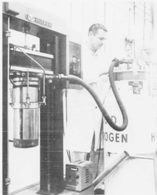
Figure 11. Instron Test Machine and Cryostat Ready for a Liquid Hydrogen Test
