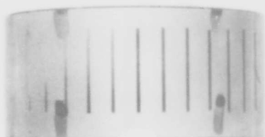
a. Unfailed Inner Race 14,000 lb Load, -1^{\circ} Angle
