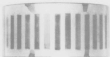
c. Unfailed Inner Race 20,000 lb Load, +5^{\circ} Angle
