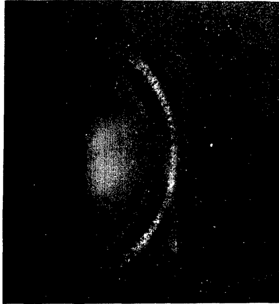
DIFFRACTION PATTERN OF TITANIUM DEPOSITED ON STEEL HEATED AT 1500°F
