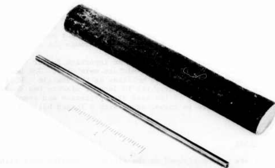
Figure 3. Photograph of as-forged Uranium Bar and finished Wire
