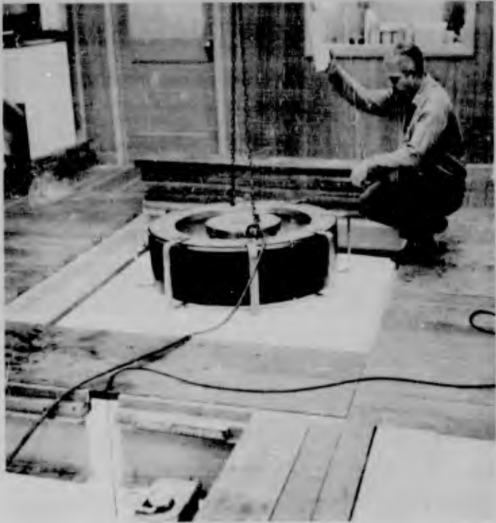
Figure 7. Flooring removed to enable positioning of large transducer.
