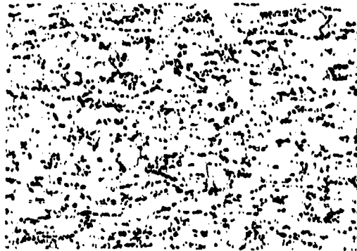
(C) LONGITUDINAL GRAIN (500x)
