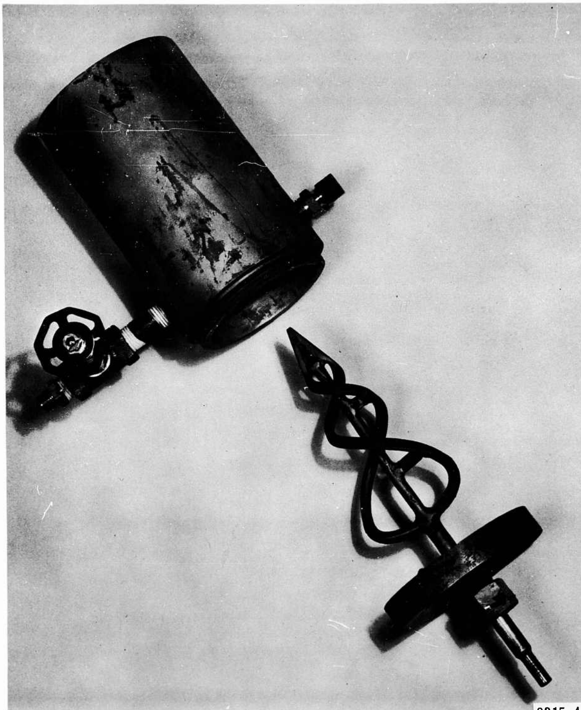
Figure XI. Experimental Conical Mixing Head. Conical Body and a Modified Helicone* Paddle.
