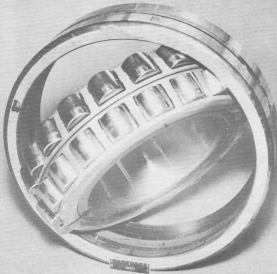
Fig. 35 Test No. 1 View of 100 mm Full Assembly Spherical Roller Bearing after Running 26.6 Hours on a Film of \text{MoS}_2 and Epoxy Binder-One Set of Rollers is Polished, The Other Set Has Picked Up a Thin Film of Lubricant
