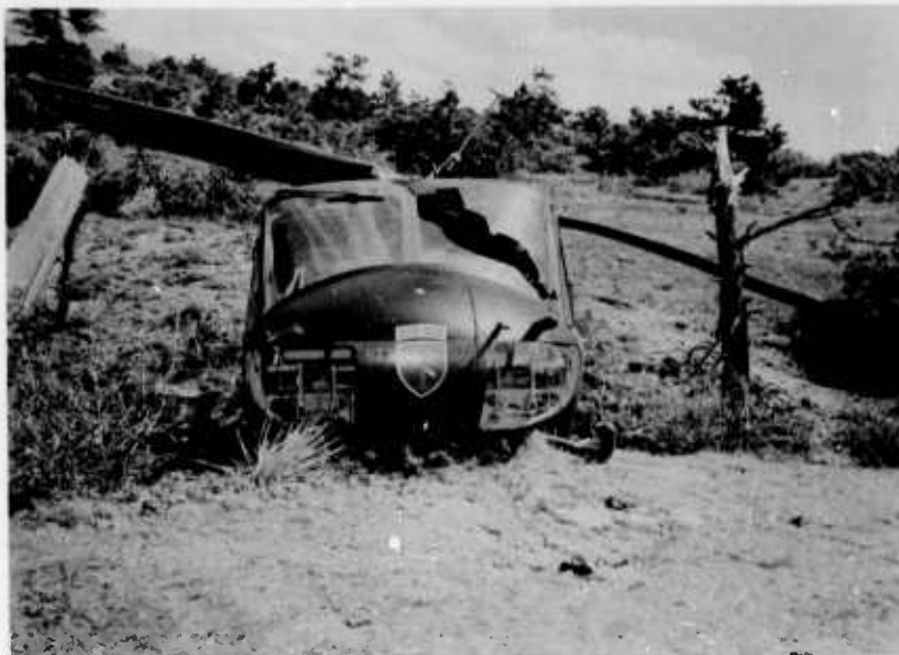
Figure 4. Front view of the helicopter showing broken plexiglas in both pedal wells and left windshield. Destruction of the main rotor is clearly shown.
