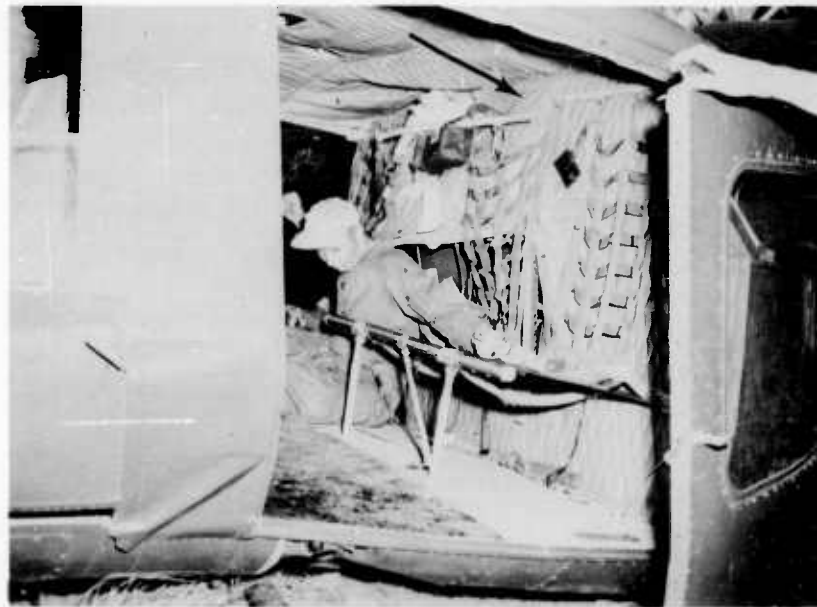
Figure 24. Posed photograph from left side of aircraft shows final position of occupant and broken seat back upper attachment (arrow).
