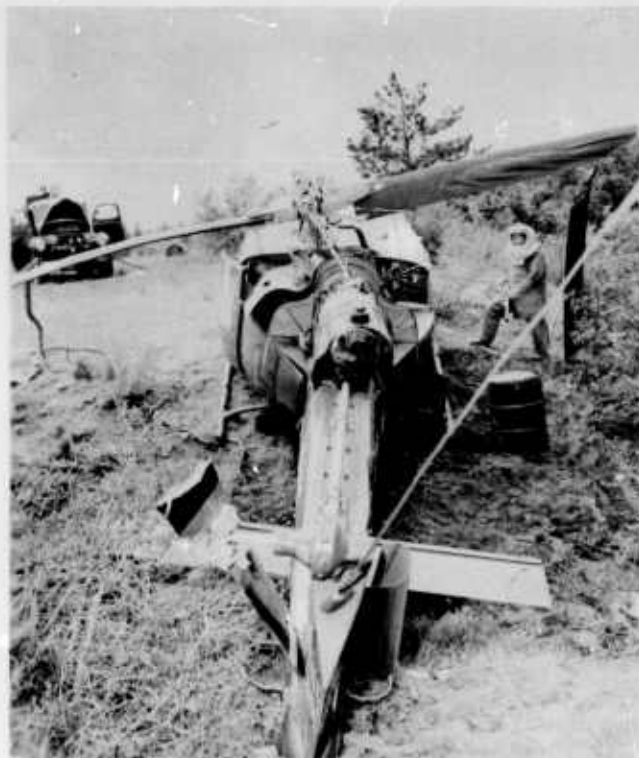
Figure 7. Rear view of helicopter showing demolished rotors and twisted tail boom.
