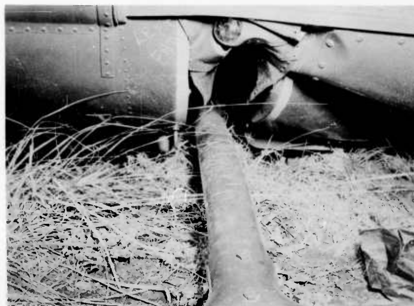
Figure 19. Left side view of aircraft showing displacement of the left forward cross tube and distortion to underside of the main cabin.
