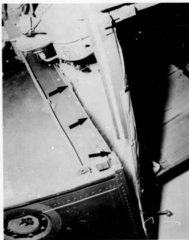
Figure 17. The forward displacement of the firewall, left side, is depicted by the arrow.
