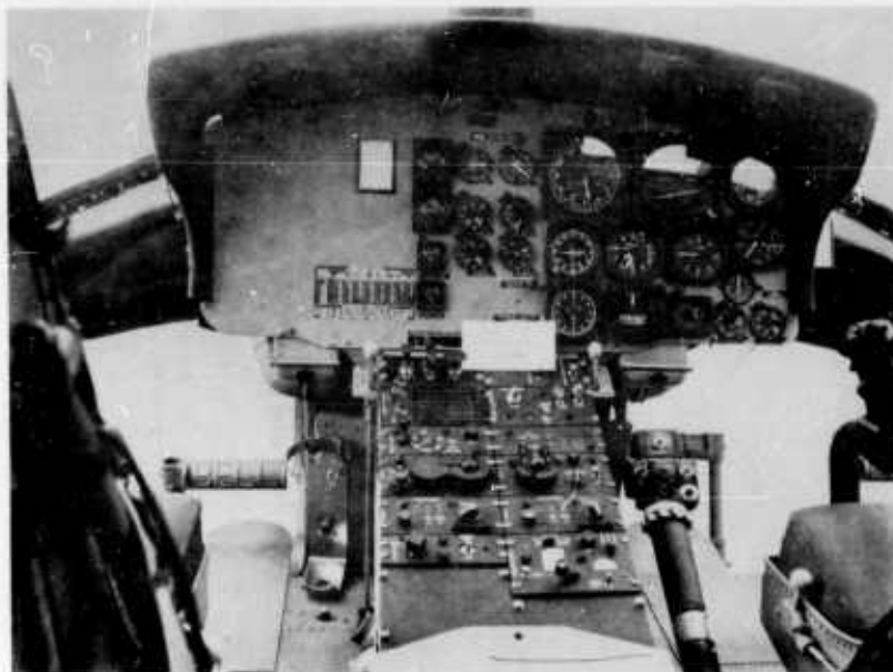
Figure 21. The intactness of the cockpit is depicted in this photo. The fire extinguisher was removed after the accident.
