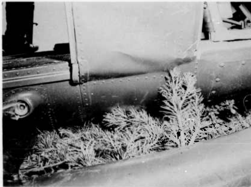
Figure 12. Side view showing distortion and impending separation of right vertical support at lower attachment.
