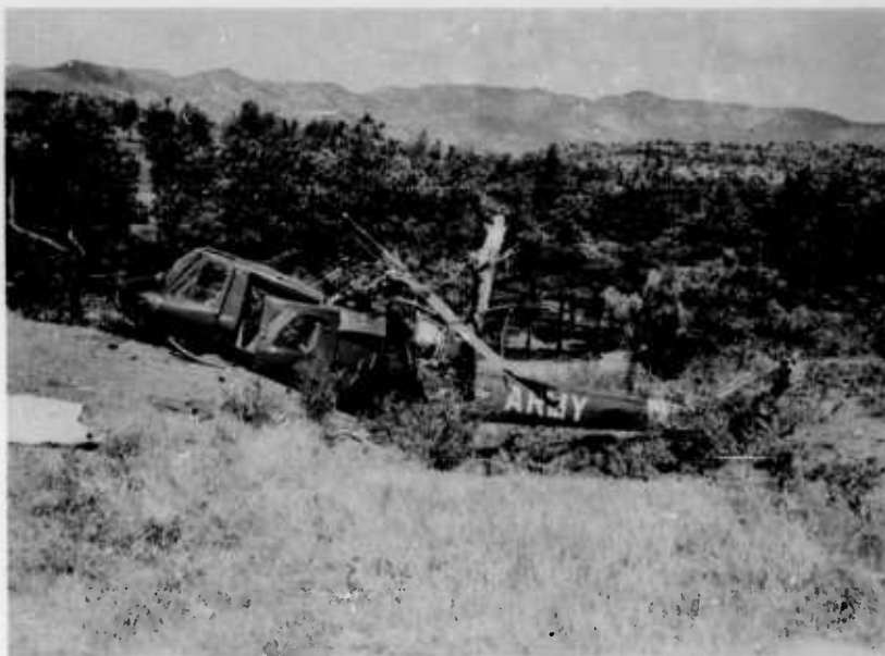
Figure 5. Side view of aircraft showing embankment struck with relative position of pine tree.
