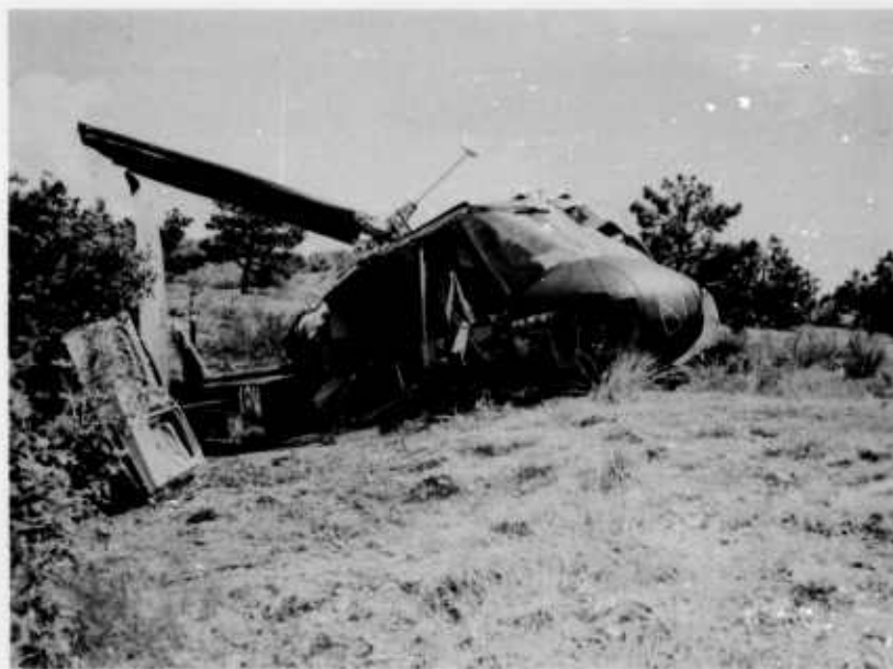
Figure 6. Right front view of the helicopter. Note the distorted right skid.
