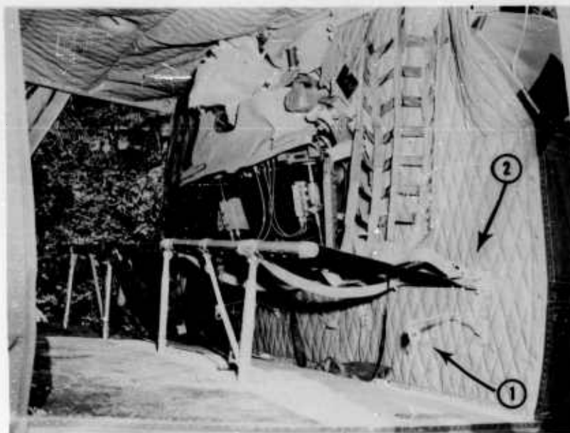
Figure 27. Arrow 1 denotes the desirable safety belt attachment. Arrow 2 depicts the manner of attachment which is normally utilized.
