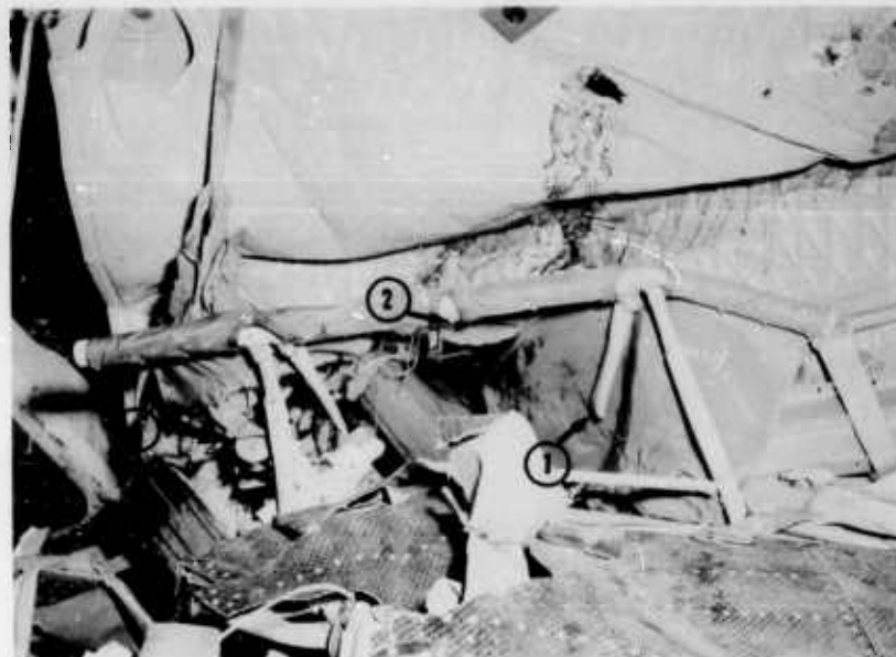
Figure 20. Failure of right rear troop seat. Note the ground handling wheels under the outboard seat. Arrow 1 indicates the broken seat spreader. Arrow 2 shows the failure of the diagonal brace. Arrow 3 indicates the position of the ground handling wheels.
