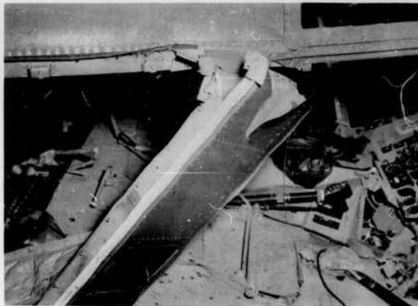
Figure 9. Side view showing failure of right vertical side support at the upper attachment to the roof structure.
