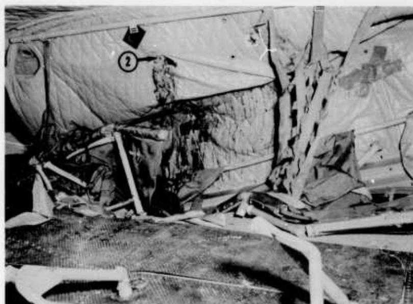
Figure 24. View of the right rear troop seat. Arrow 1 shows where the seat pan tore across the ground handling wheels. Arrow 2 indicates the structural member that pierced the bulkhead, injuring the occupant of the inboard seat.
