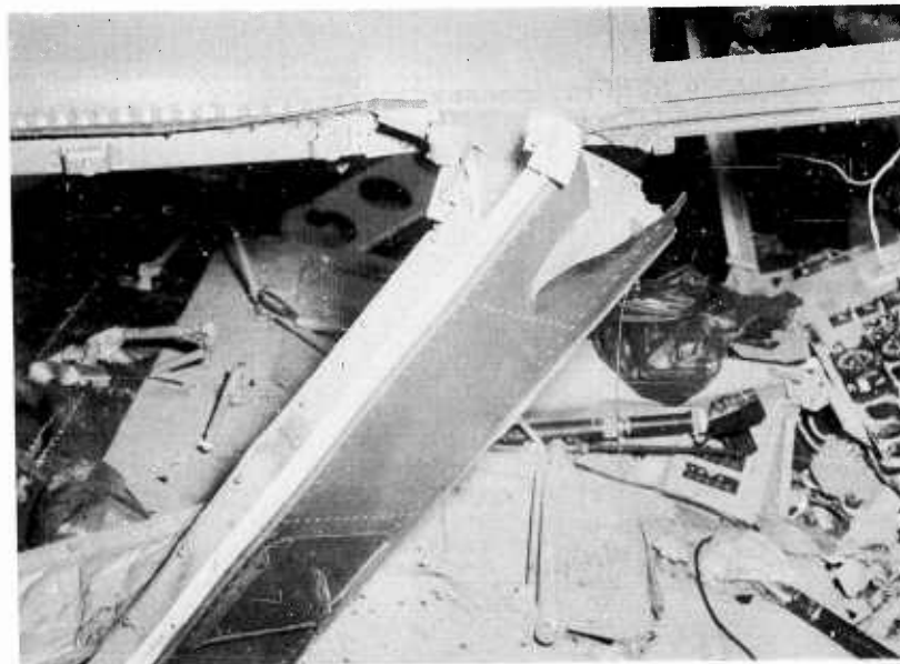
Figure 15. The top of the right side was supported by the wiring, Accident "D".
