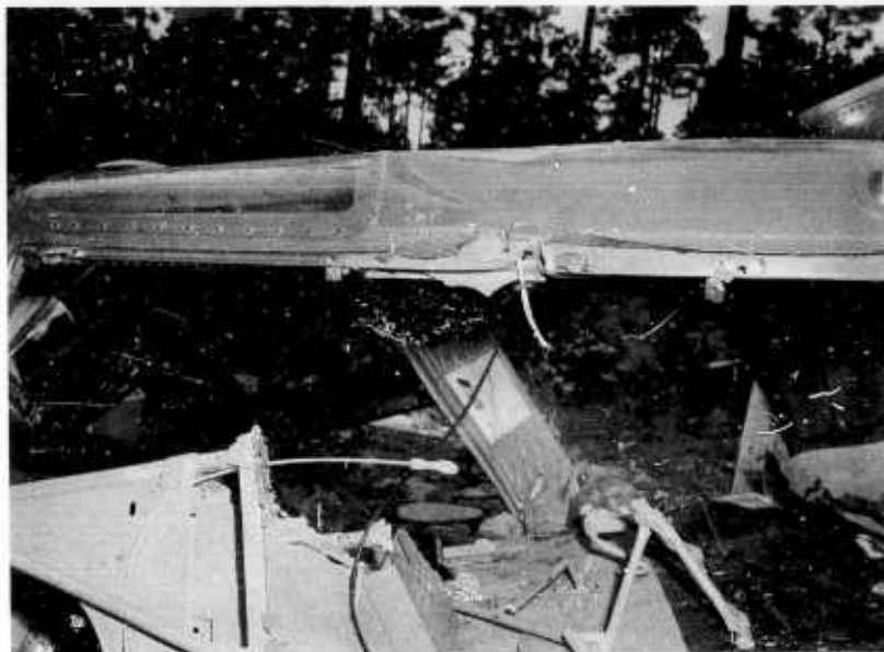
Figure 12. The top left vertical side support was torn completely free in Accident "D".
