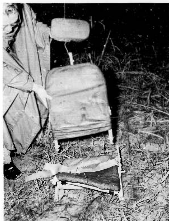
Figure 49. Damaged crew chief's seat.
