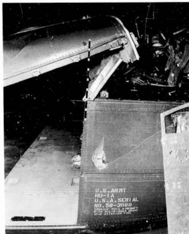
Figure 18. Partial failure occurred on the top of the support, left side, in Accident "E".
