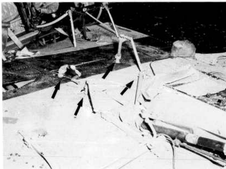
Figure 48. Crew chief seat failure in Accident "D". The arrows depict failures of the leg structure.
