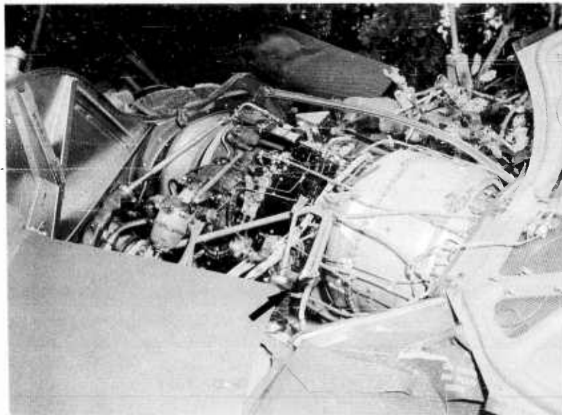
Figure 33. The arrow depicts a partial failure in the engine mounts in Accident "D".
