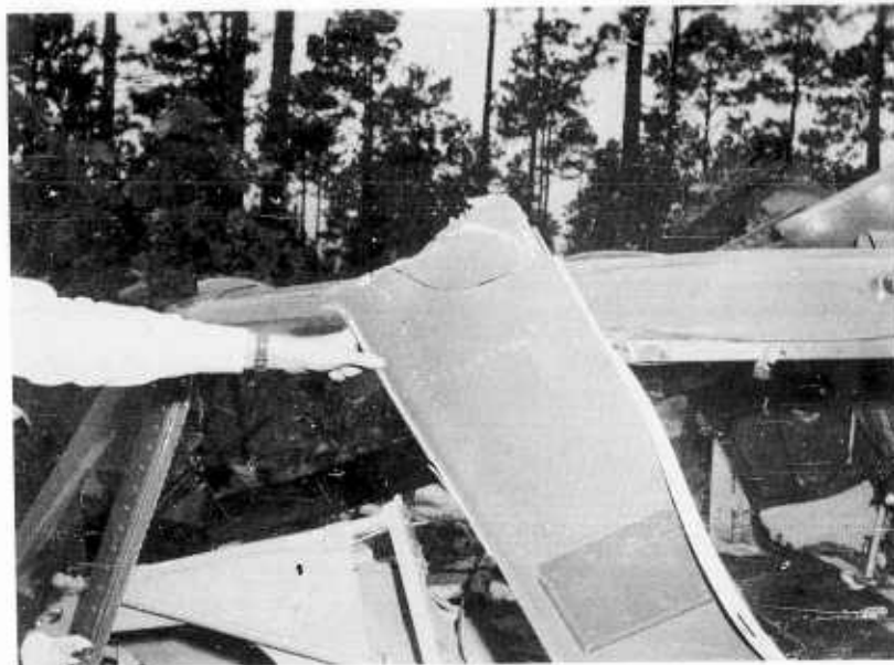
Figure 14. Side view of the torn free support in Accident "D", left side.
