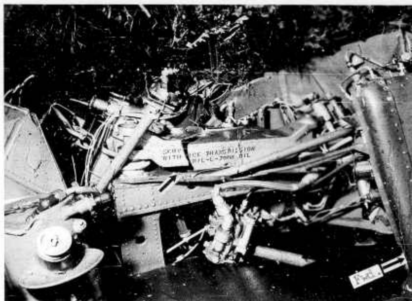
Figure 25. The arrow depicts the failure in the transmission mount which occurred in Accident "A". The transmission, mast, and rotor assembly were partially torn free as a unit.
