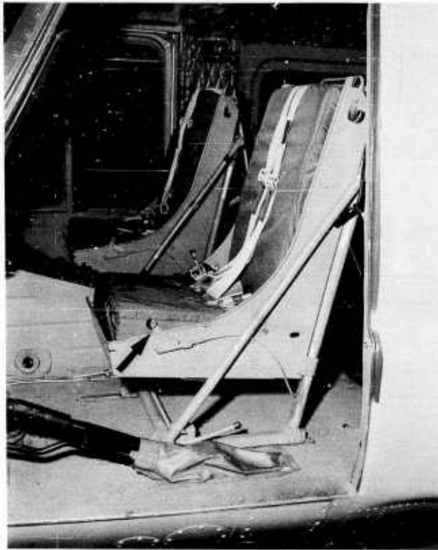
Figure 35. A side view of the pilot's seats. The inertia reel manual locking lever is conveniently located on the side of the seat pan (arrow).
