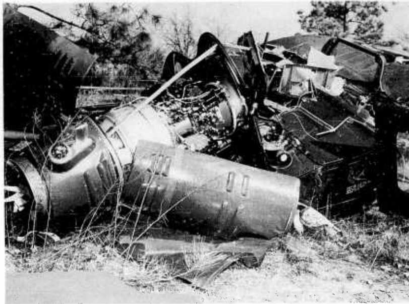
Figure 32. A partial failure in the engine mounts occurred in Accident "B".
