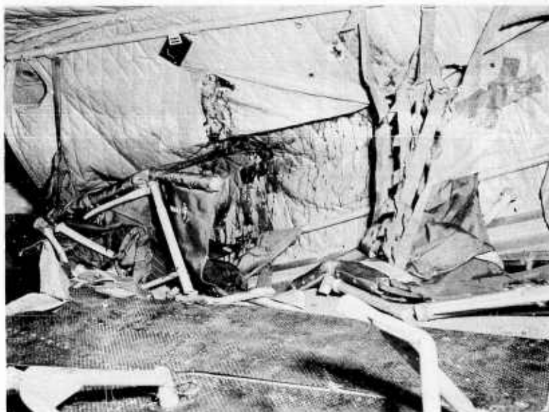
Figure 52. The right side cabin seats in Accident "D" were broken.
