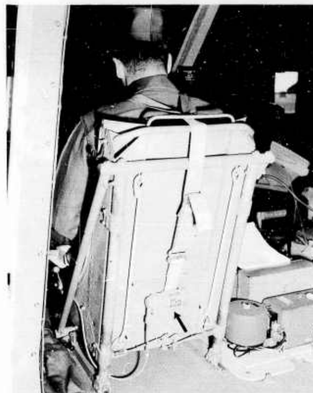
Figure 37. The arrow depicts the inertia reel attached to the rear of the seat. Note the width of the shoulder harness guide at the top of the seat. This is considered excessive.
