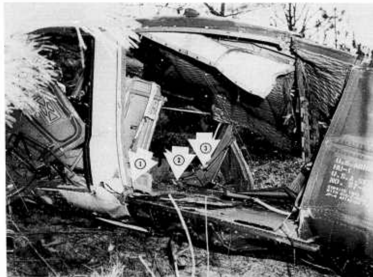
Figure 7. Left side support failure in Accident "B". Arrow 1 depicts the failure on the bottom of the left side support. The top remained attached. Arrow 2 depicts the broken seat attachment, Arrow 3 shows the bent seat tube support.
