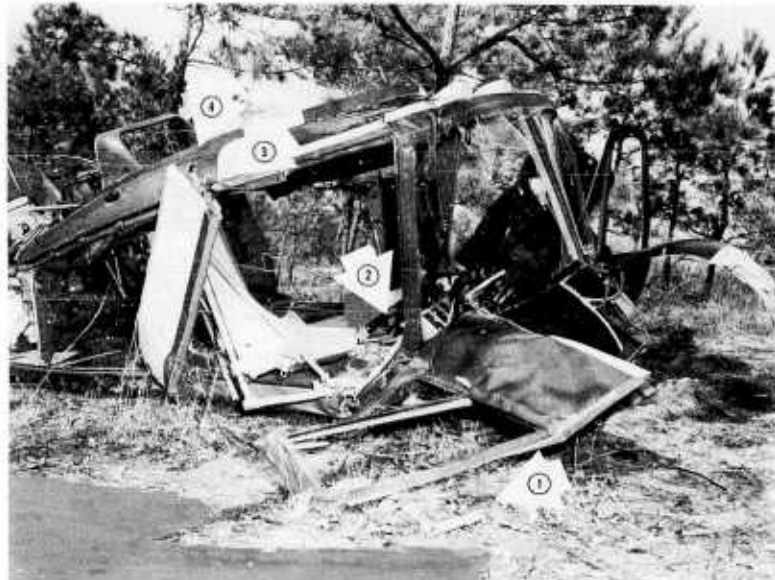
Figure 6. Right side support failure in Accident "B". The upper right side support (arrow 3) was torn free, the bottom also failed. Arrow 1 depicts the pilot's right anti-torque pedal, Arrow 2 damage to collective pitch, while Arrow 4 denotes a hole in the roof caused by the pilot's seat as the roof collapsed.
