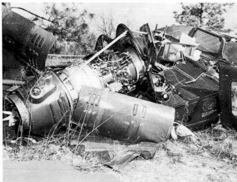
Figure 26. The entire unit was torn free when the blades contacted a tree in Accident "B". The arrow depicts the area normally occupied by the transmission.
