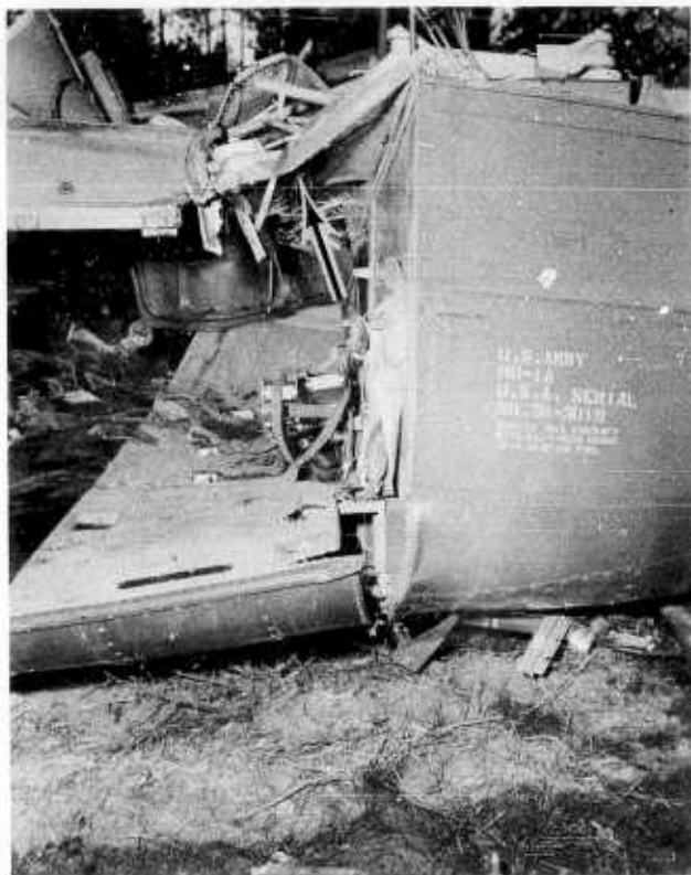
Figure 24. The forward displacement of the aft roof support is depicted by the arrow, Accident "D".
