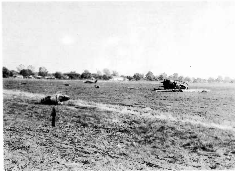
Figure 31. The arrow depicts the engine, torn free, in Accident "A".
