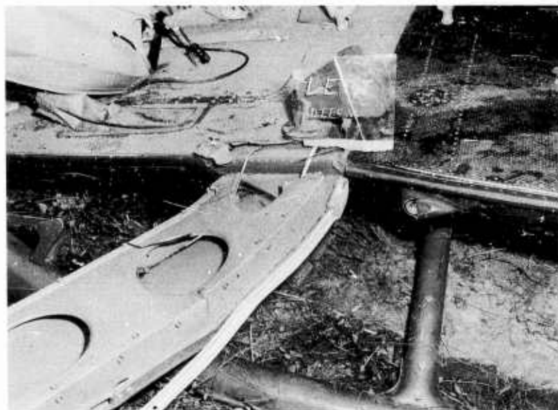
Figure 12. The top left vertical side support was torn completely free in Accident "D".
