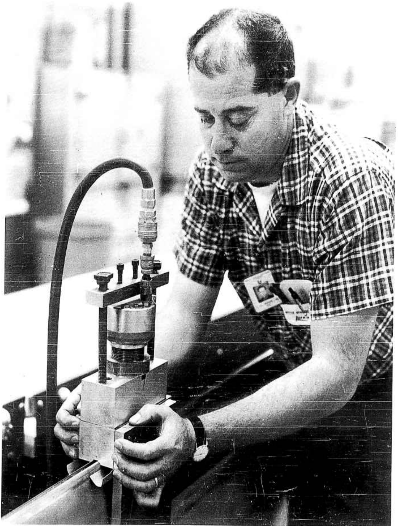
WORK AID USED TO CUT SLOT IN BLADE
