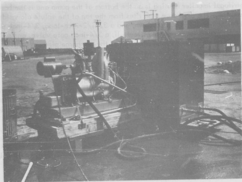
Figure 7. Snow-disposal equipment; note hose for circulating heated coolant through melter coils.
