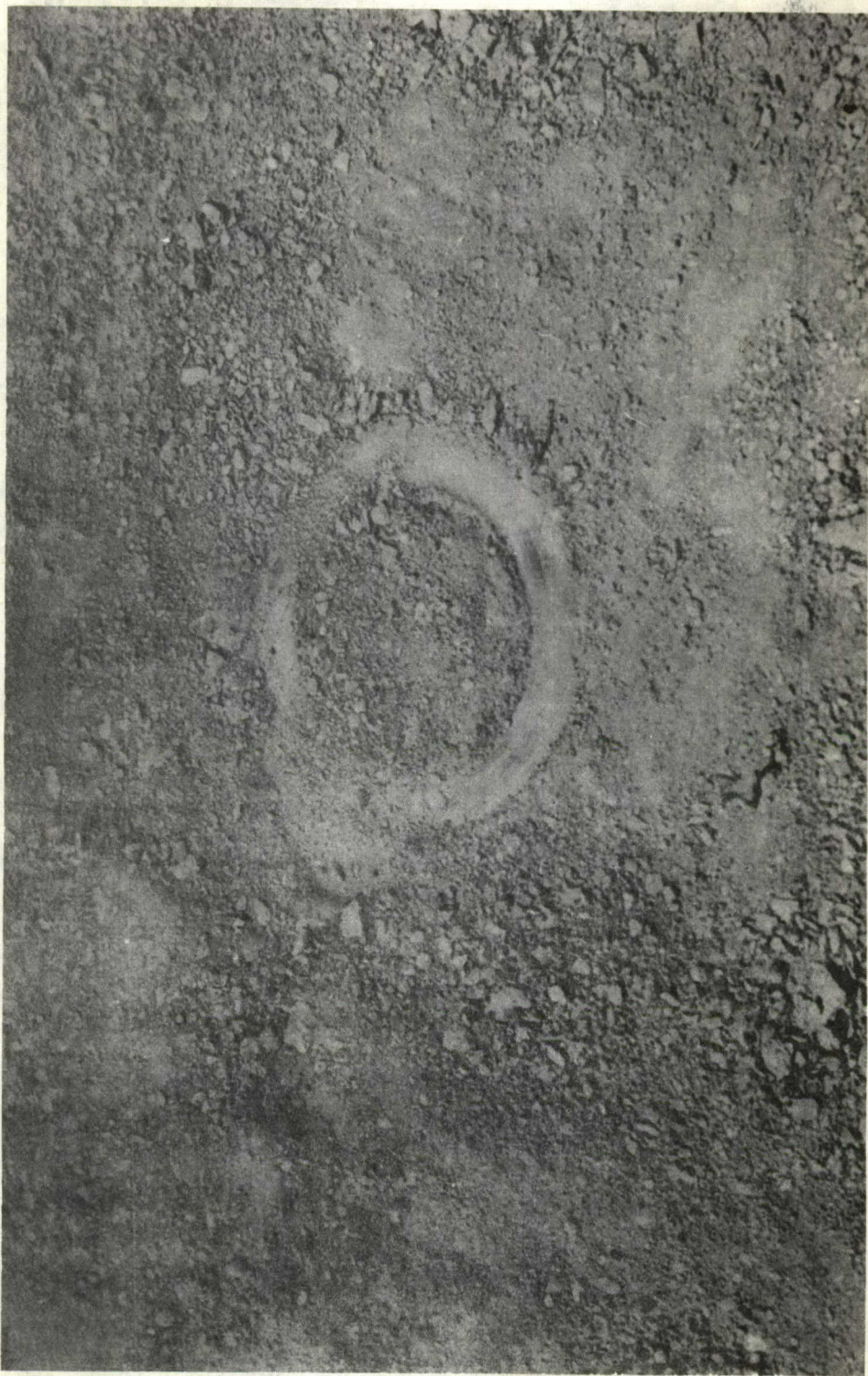
Fig. 4 SHEAR ANNULUS IMPRESSION ON HARD SURFACE, SILT COURSE, WES, VICKSBURG, JUNE, 1964.
