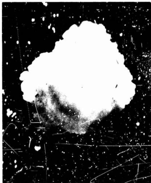
Fig. 4.2—Particles collected by a differential fall-out collector. (Note darkened area around the radioactive particle.)
