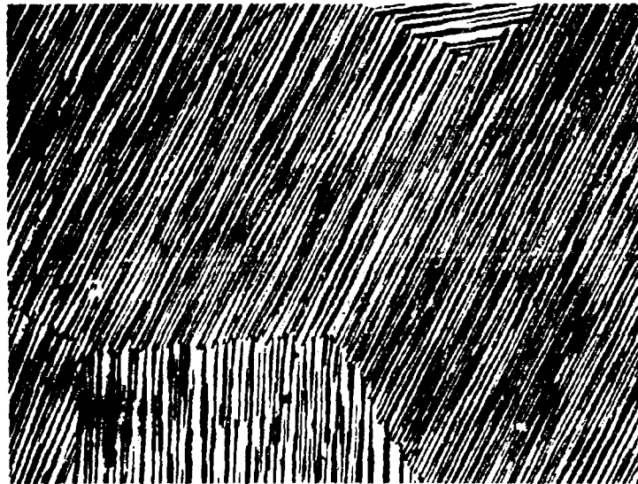
Figure 19b. Hf-C (13 At% C) Sample from Figure 19a, Re-equilibrated at 2300°C and Quenched. X150 \alpha -Hf-Solid Solution with Oriented Precipitation of Monocarbide Formed During Cooling.
