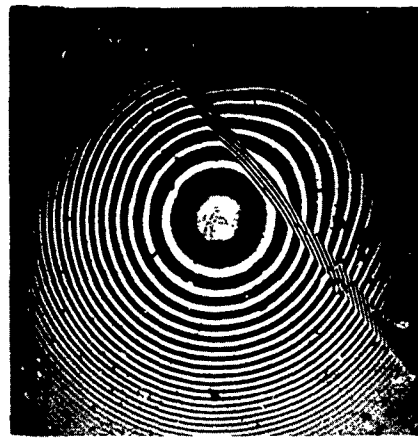
Fig. 4 Twin strip on the (0001) plane of a Zn crystal containing 0.0005% Al. 165x.
