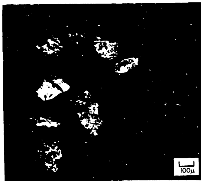
Figure G.1 (e) Photomicrograph DT D-050 +150 mesh (wet sieved) (105 to 149μ)
